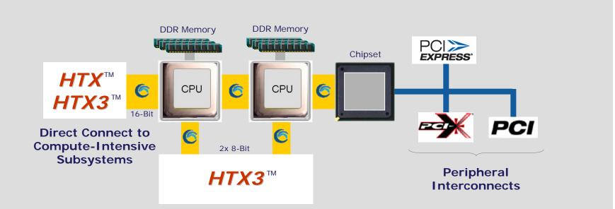
With its Unique Architectural and Performance Edge over General Purpose Interconnects, HTX is an Ideal Complement to PCI-Class Slot Connector Interfaces
