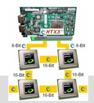
Allows HTX Subsystem to Connect Directly to 2 CPUs Supports New-Generation System Functionality
