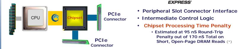
HTX Delivers 55% Lower Latency per Transaction Due to Absence of Intermediate Control Logic and Multiplexing
