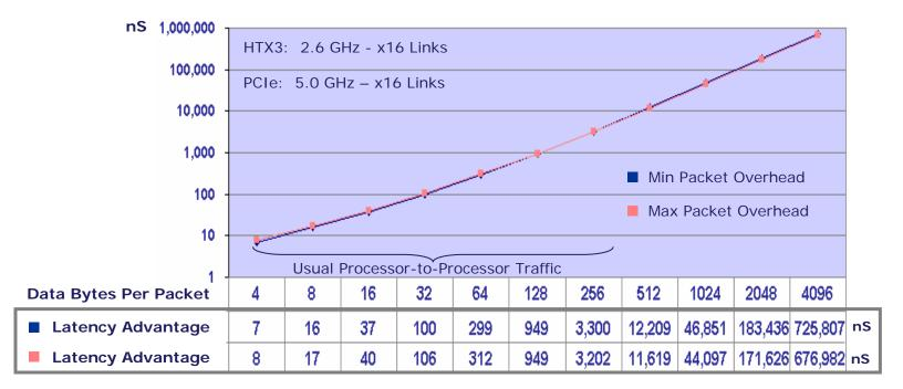
The results take into account PCIe's 20% clock recovery, packet payload and 55% chipset overhead penalties. HTX's Priority Request Interleaving, if applicable, will add to HTX's total latency advantage
