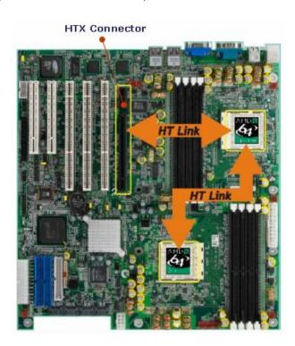
System manufacturers may choose locations other than slot 6 for the HTX connector that they may deem more suitable for specific market targets and applications, provided that proper routing and signal integrity guidelines are complied with
