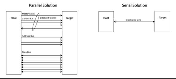
Figure 1: Parallel vs. Serial Clock Implementation
