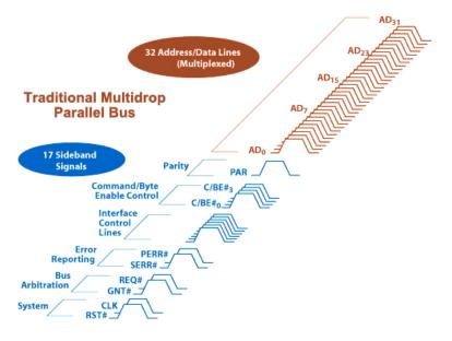
Figure 3: 32-bit Wide Parallel PCI Bus
