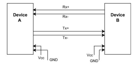
Figure 4: Ethernet Interface Signals
