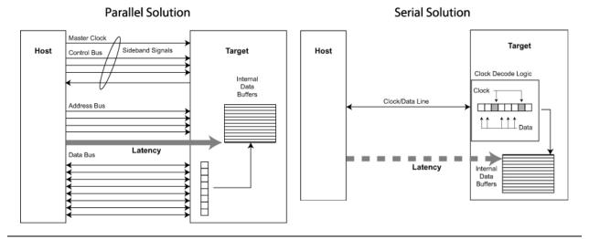
Figure 2: Parallel vs. Serial Clock Latency
