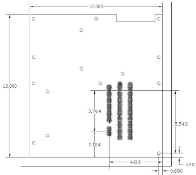
Figure 7. EATX Motherboard with HyperTransport™ Connector in Slot 6 Position
