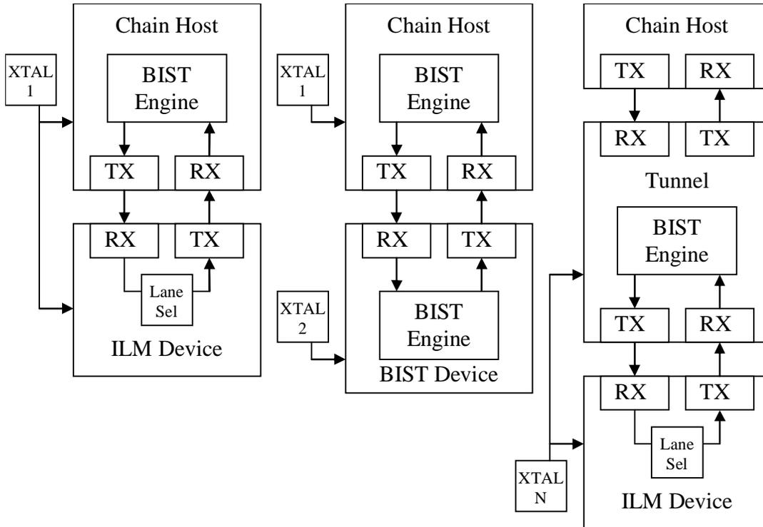
**Figure 22. Link Test Topologies**
