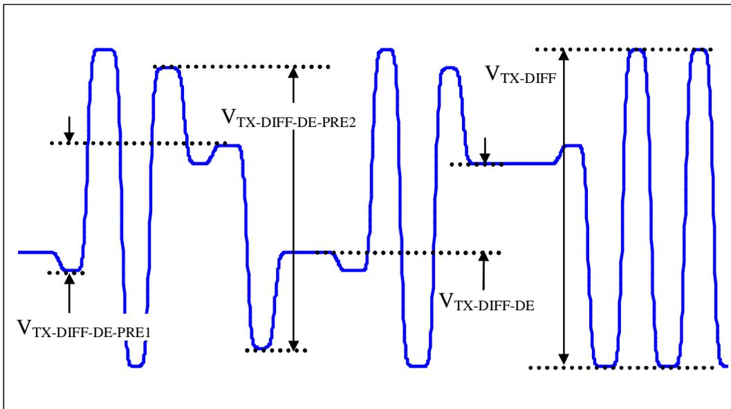
**Figure 52. Transmit with pre- and post-cursor de-emphasis**
