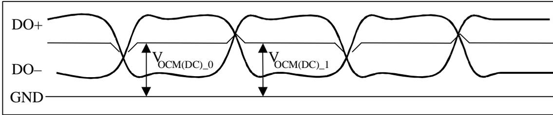
Figure 34.  $V_{OCM(DC)}$
