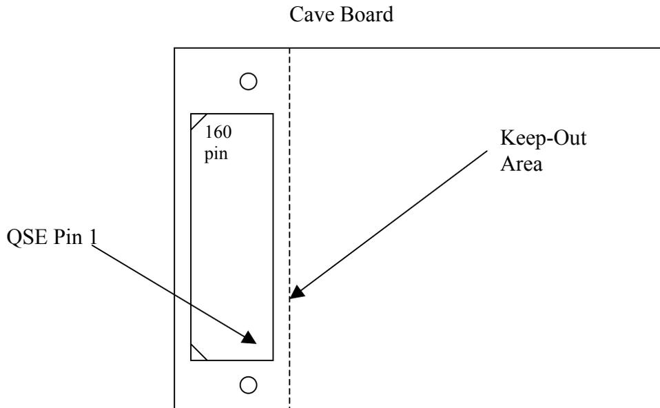
For HT 2.0 operation, only populate the connectors on the bottom of a normal cave board.
