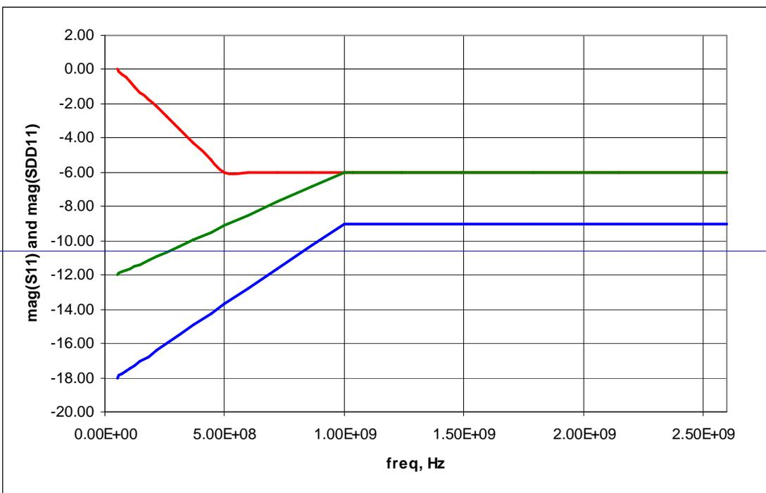
**Figure 58. Receiver return loss mask**
