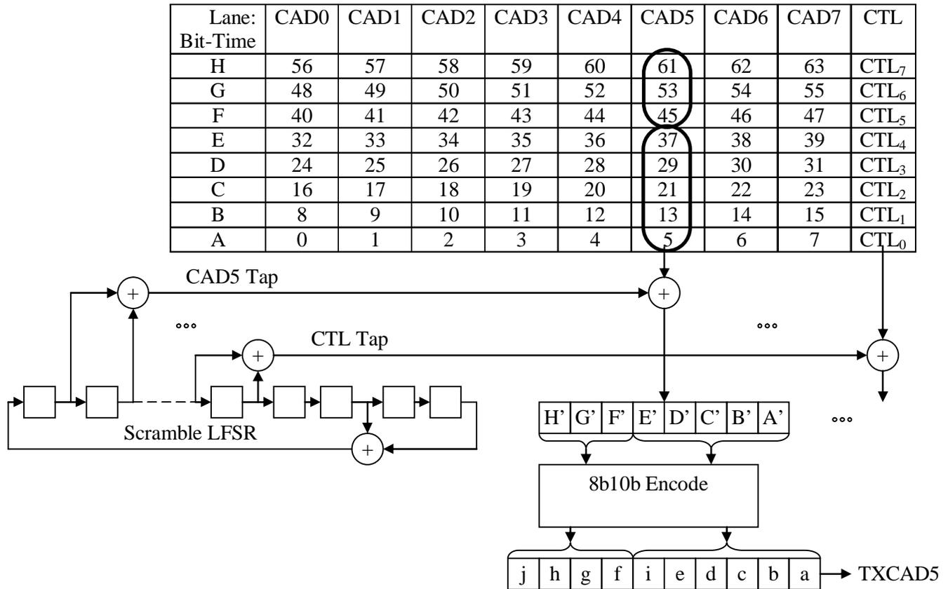
Figure 4. Gen3 Transmitter Order of Operations
