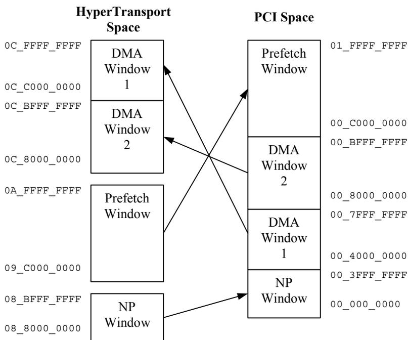
Figure 8. **DMA-Memory Window Remapping**
