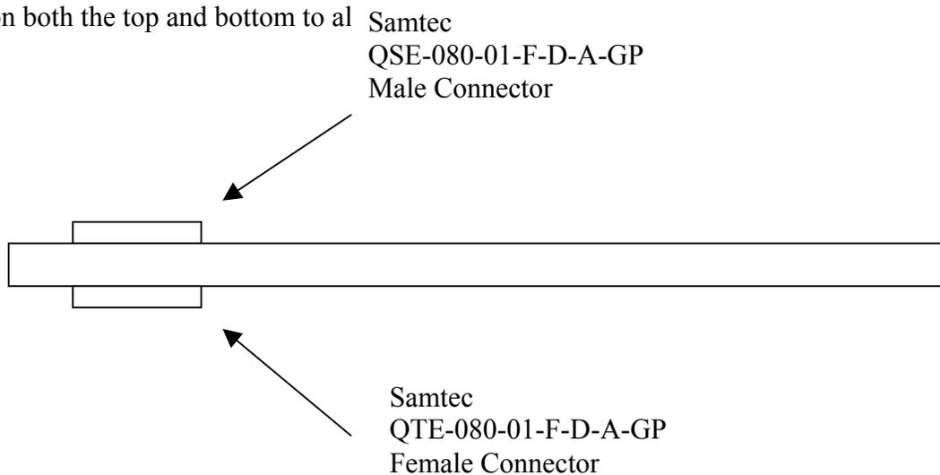
(For reference the SAMTEC QTE-080-01-F-D-EM2-GP is the board edge mounting connector that mates with the topside DUT connector. This part may be useful for evaluation boards for cave devices that want to plug in to a DUT option slot on a host evaluation card that fits in a standard form factor ATX case.)
