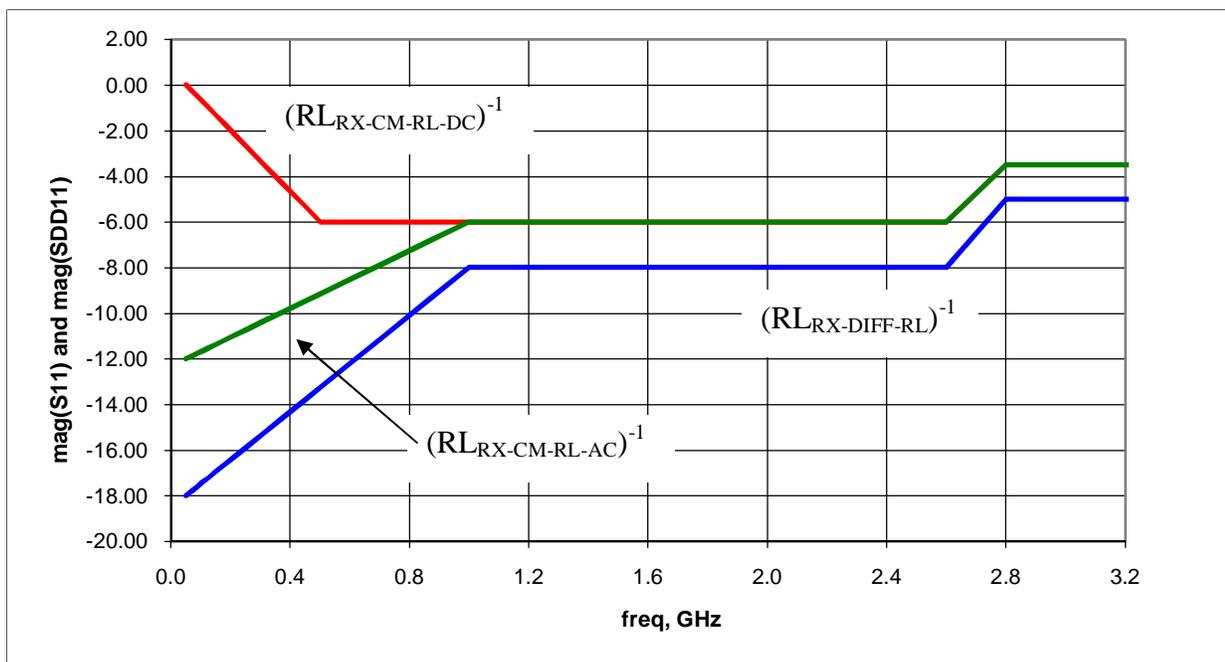
**Figure 58. Receiver return loss mask**
