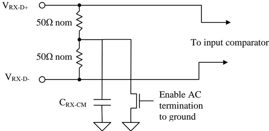
Figure 59. Receiver input termination
