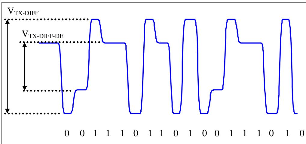
**Figure 51. Differential transmitter post-cursor de-emphasized waveform**
