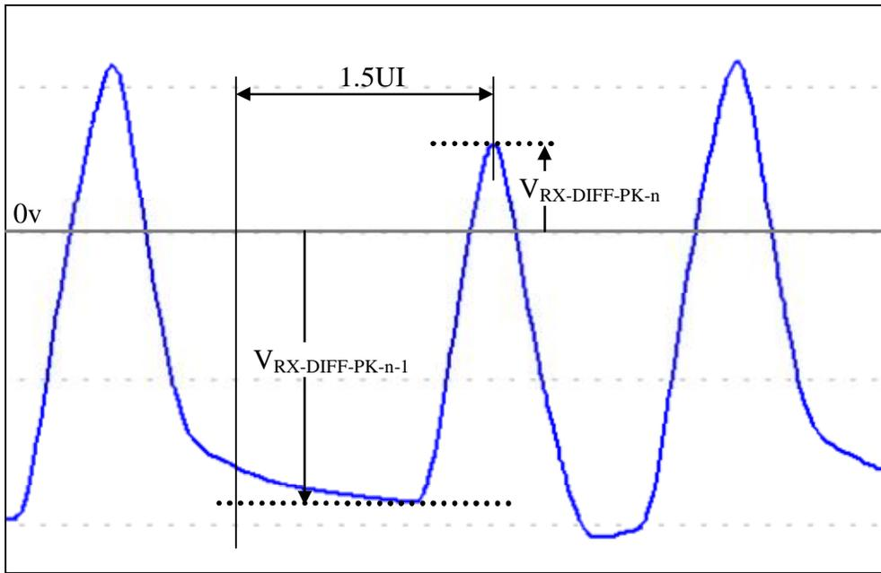
Figure 61. Receiver adjacent bit ratio
