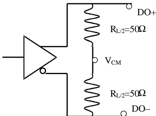
**Figure 31. DC Output Reference System Load**
