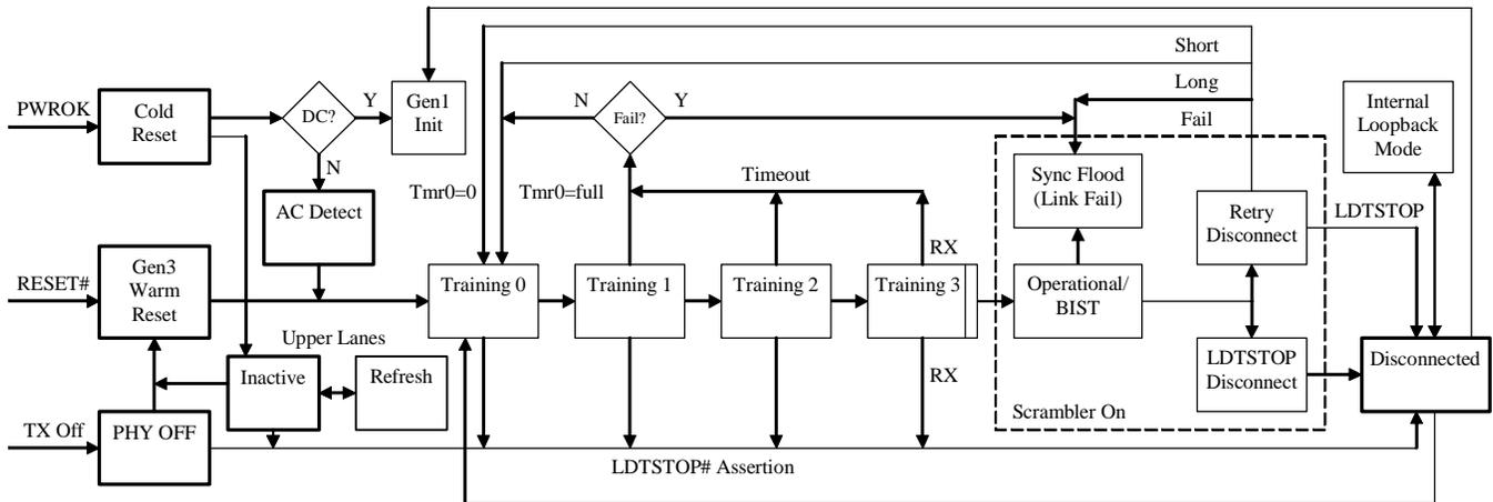
Figure 16. Link State Diagram
