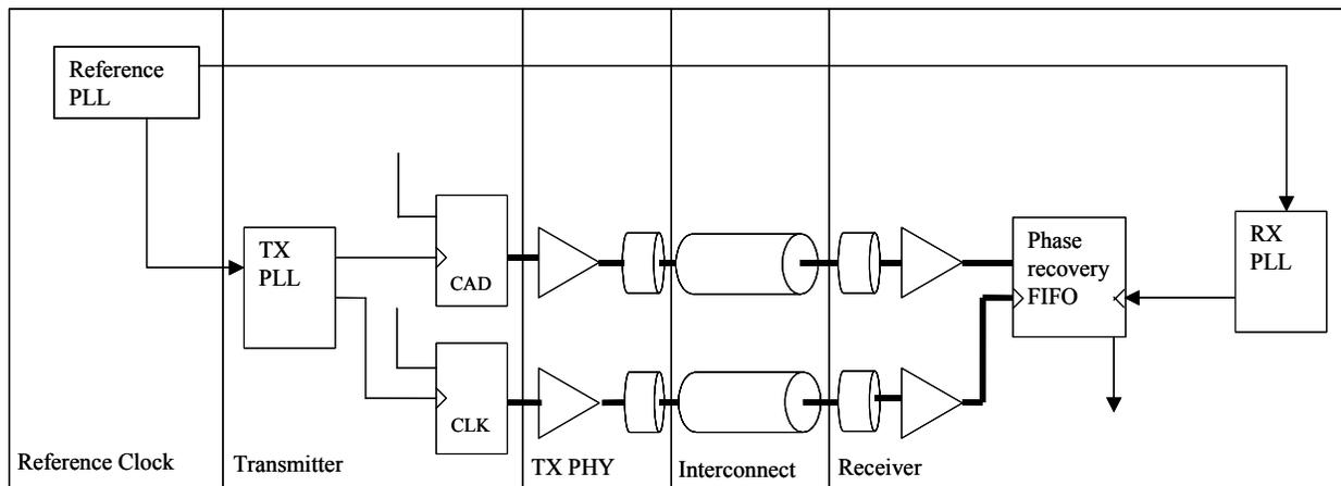
Figure 30. Representative Transmitter and Receiver
