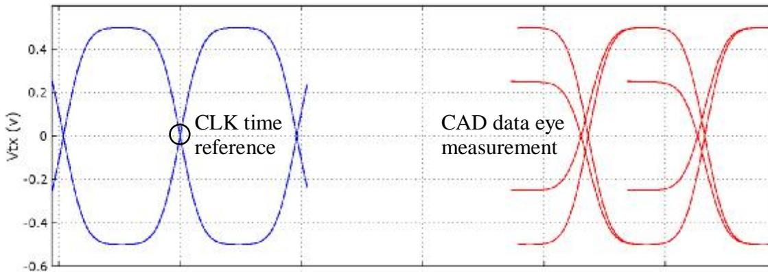
**Figure 54. CLK to CAD ideal eye with -6dB of de-emphasis**
