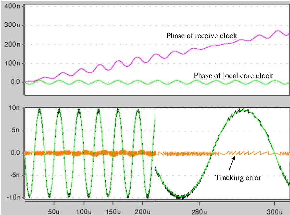
Figure 65. Phase tracking across receiver sync-fifo
