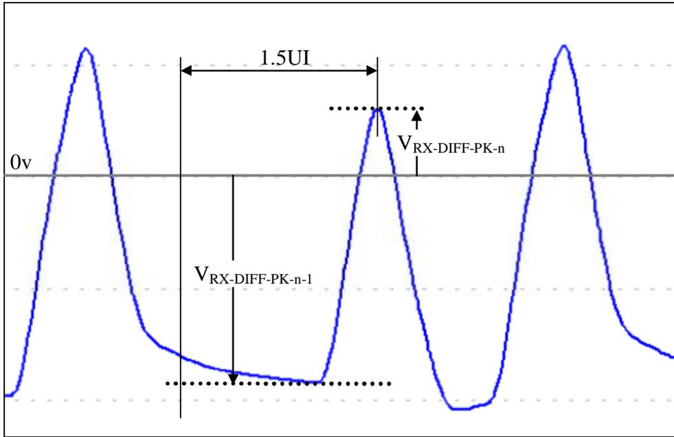
Figure 61. Receiver adjacent bit ratio
