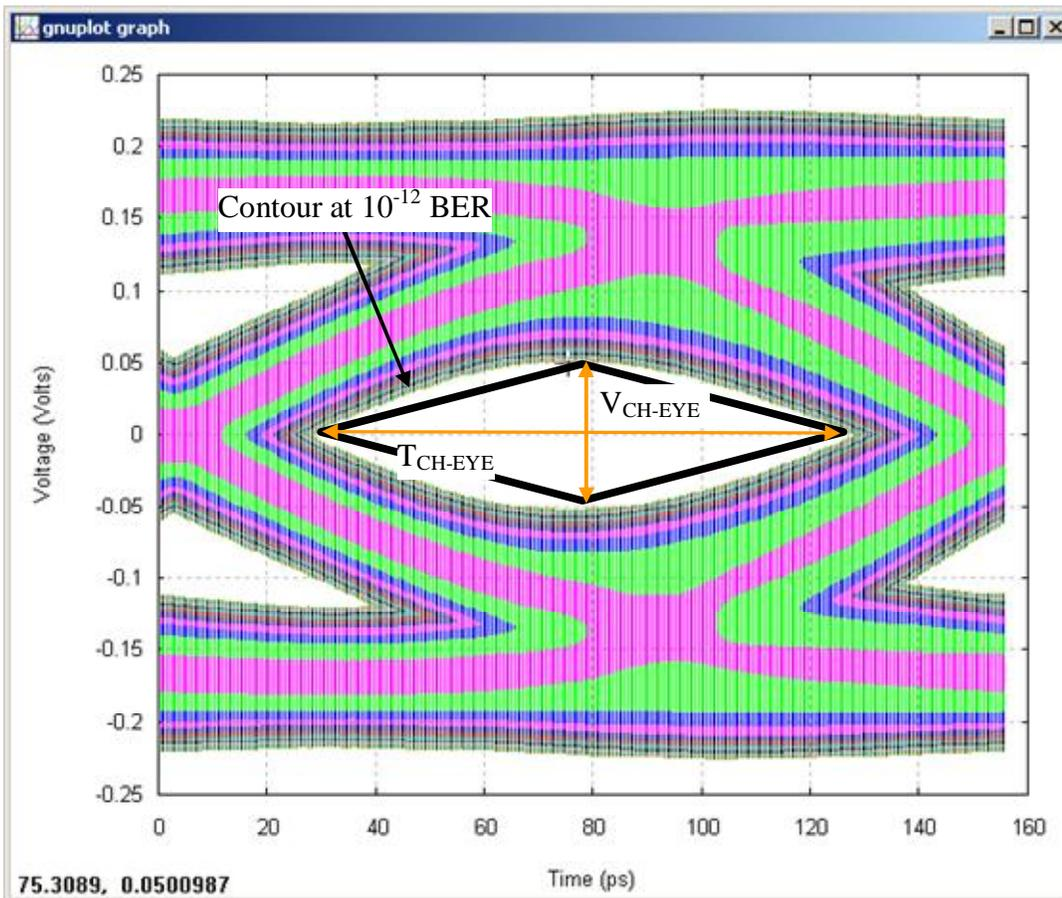
Figure 57. Channel compliance eye diagram
