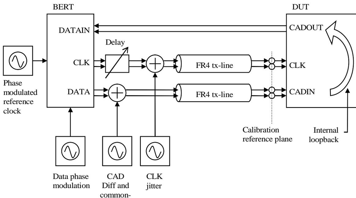
**Figure 63. Receiver input compliance test setup**
