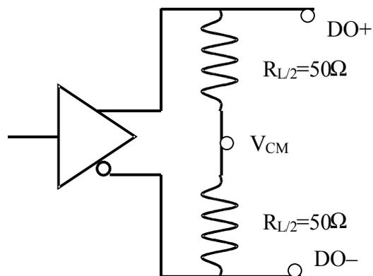
Figure 19. DC Output Reference System Load
