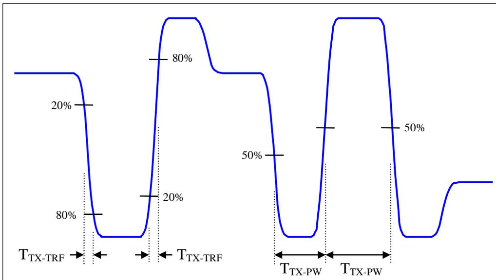
Figure 53. Rise time, fall time and pulse width measurements
