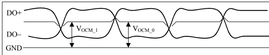
**Figure 21.**  $V_{OCM}$  DC
