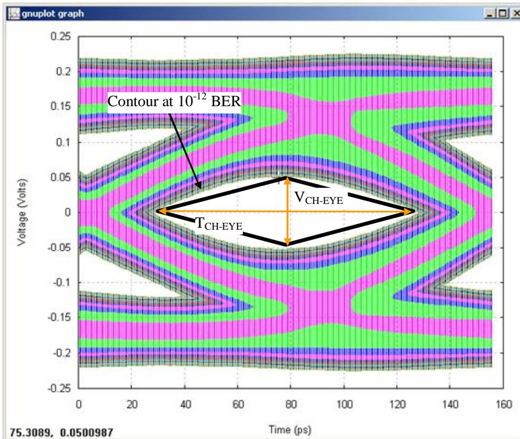
**Figure 57. Channel compliance eye diagram**
