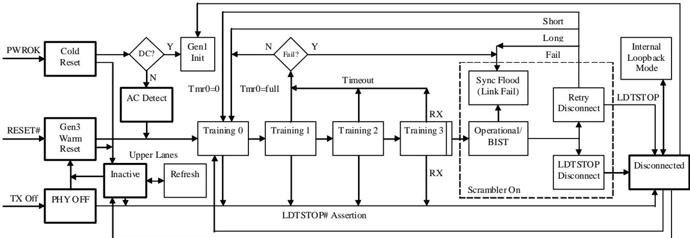
Figure 17. Link State Diagram
