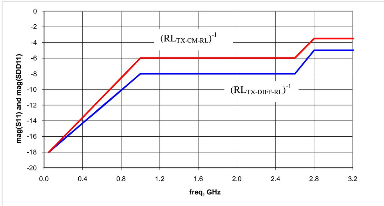
Figure 50. Transmit return loss mask
