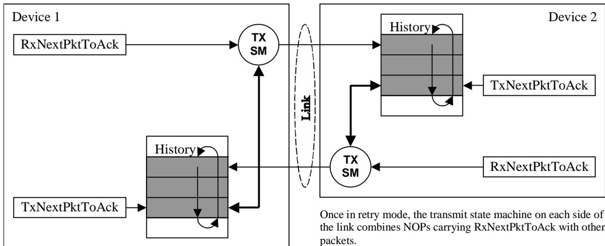
Once in retry mode, the transmit state machine on each side of the link combines NOPs carrying *RxNextPktToAck* with other packets.
