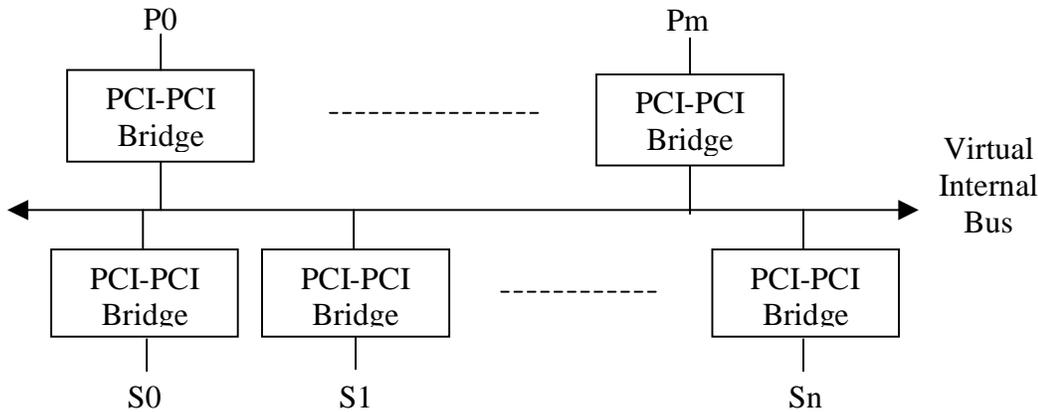
**Figure 29. Logical Model of a Switch**
