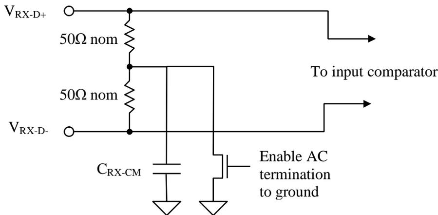
Figure 59. Receiver input termination
