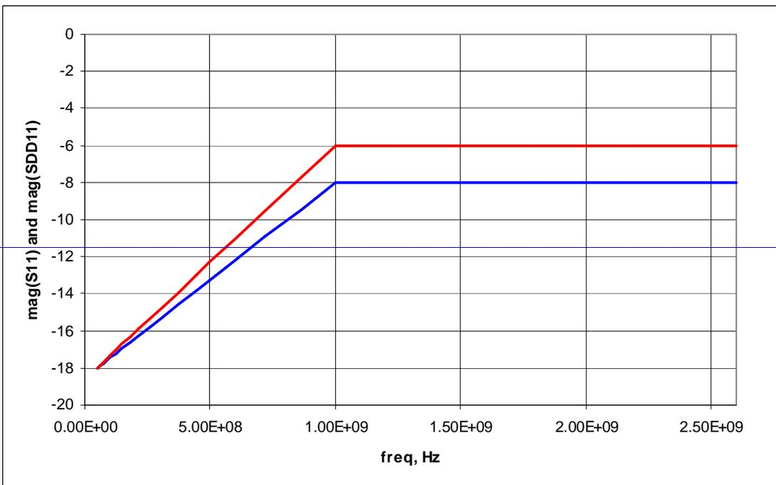
**Figure 50. Transmit return loss mask**
