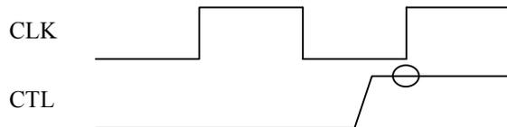
**Figure 9. Sync Sequence Timing for Link Initialization**
