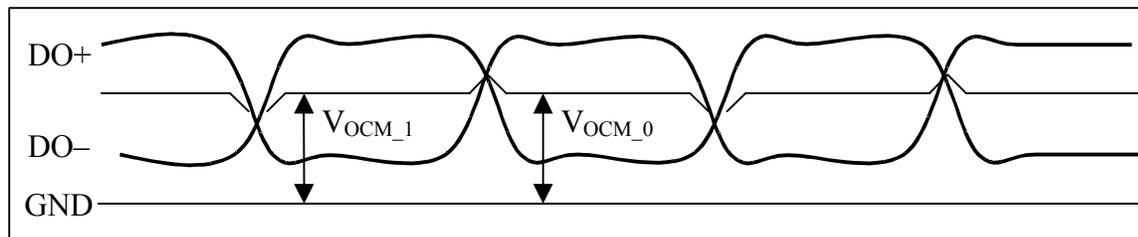
**Figure 21.  $V_{OCM}$  DC**
