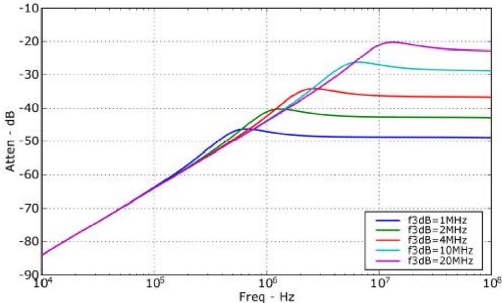
**Figure 49. System reference clock jitter rejection**
