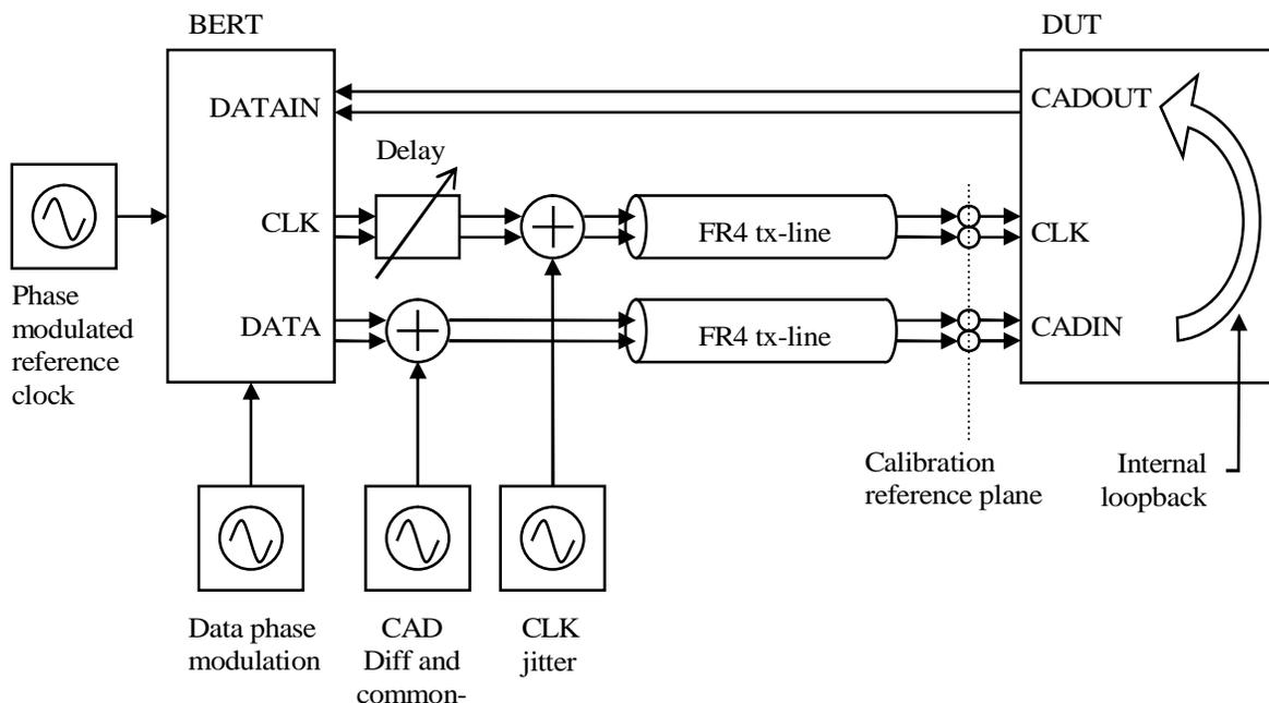
**Figure 63. Receiver input compliance test setup**
