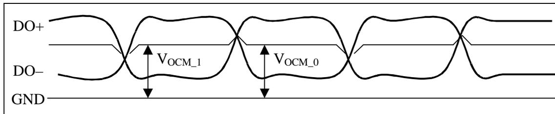
**Figure 19.  $V_{OCM}$  DC**
