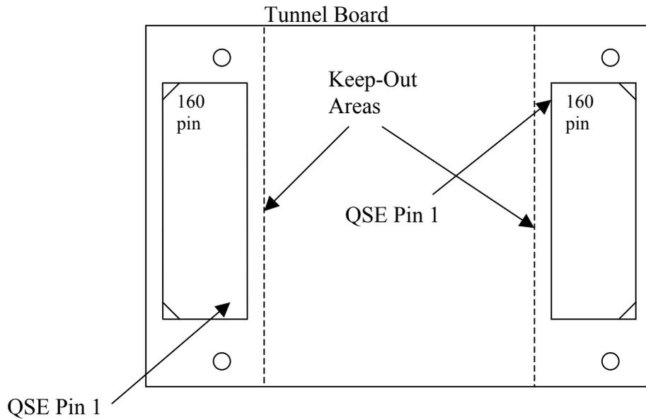
For HT 2.0 operation, only populate the connector on the bottom of the tunnel on the side that will connect to a host, and on the top of the side that will connect to a cave or another tunnel. (Note that for full testing of the tunnel two boards must be made to ensure both ports work correctly when towards the host.)
