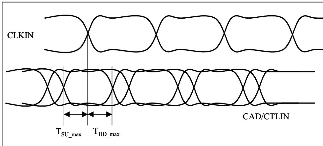
Figure 27.  $T_{SU}$  and  $T_{HD}$
