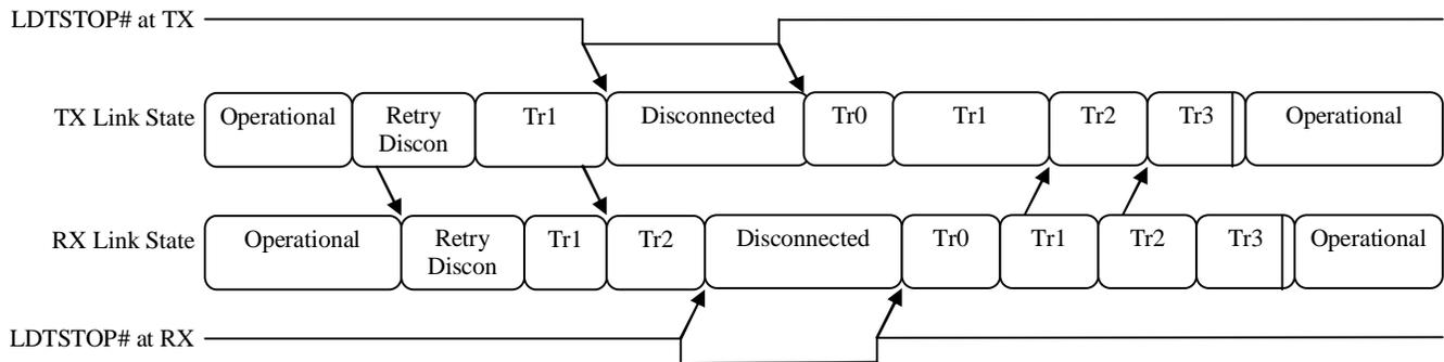
**Figure 20. Example LDTSTOP Disconnect Sequences**
