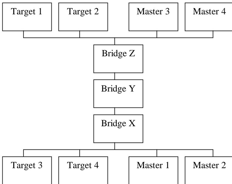
**Figure 26. Example PCI System**
