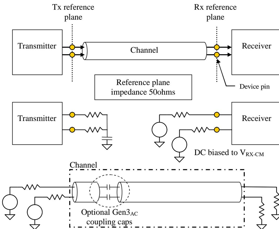
Figure 48. Measurement methodology of HyperTransport™ link components
