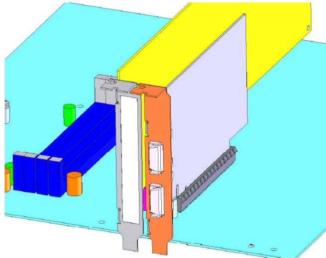
Figure 3. 3U System with Vertically Mounted HT Daughtercard
