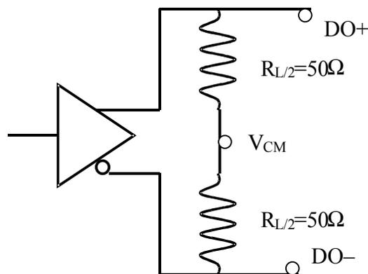
**Figure 13. DC Output Reference System Load**
