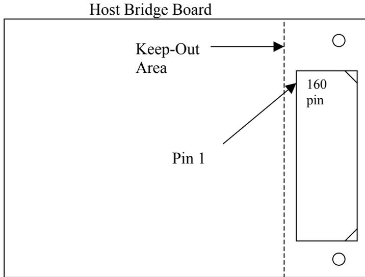
For HT 2.0 operation, only populate the connectors on the top of a normal host bridge board.
