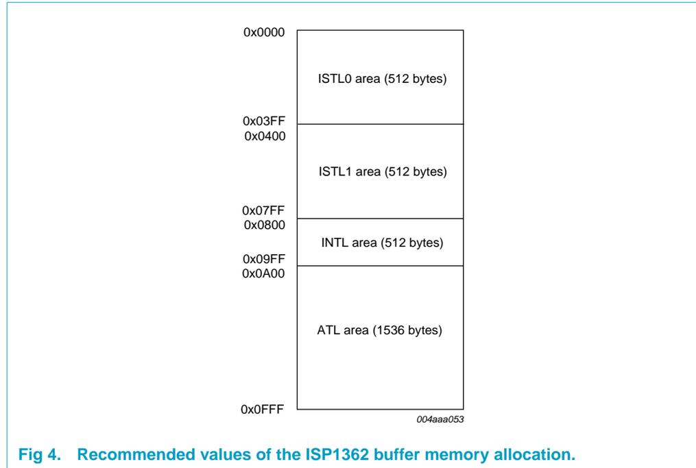
**Fig 4. Recommended values of the ISP1362 buffer memory allocation.**
