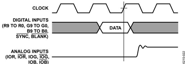
Figure 22. Video Data Input/Output
