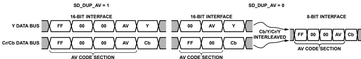
Figure 30. AV Code Duplication Control (64-Lead LQFP Only)
