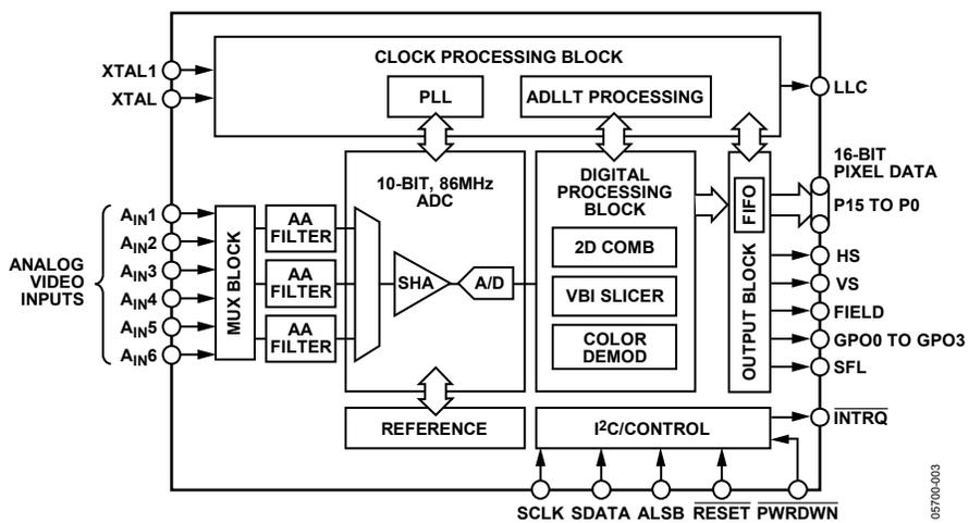
Figure 2. 64-Lead LQFP Functional Block Diagram
