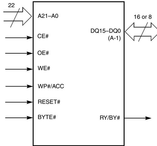
**Figure 5.3** S29GL064N Logic Symbol
