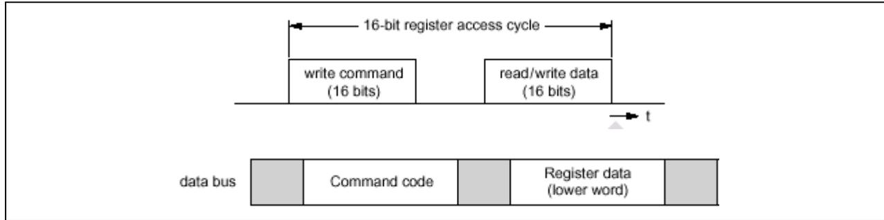
Figure 3-1: 16-Bit Register Access Cycle
