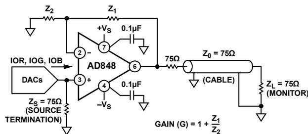
Figure 27. AD848 As an Output Buffer
