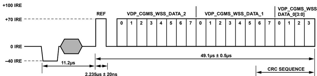
Figure 43. CGMS Waveform
