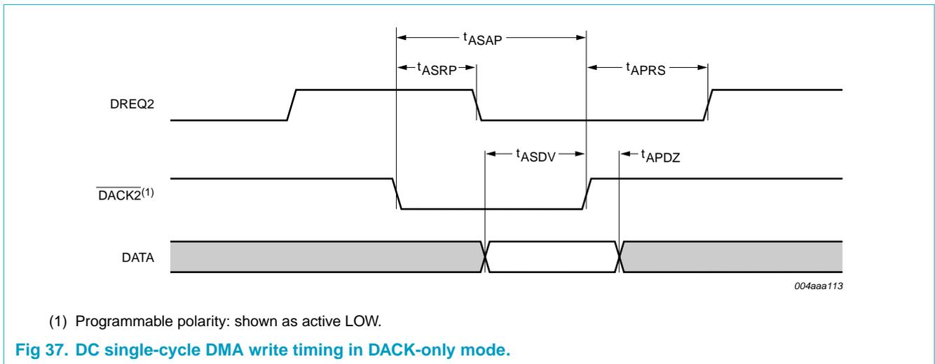
Fig 37. DC single-cycle DMA write timing in DACK-only mode.
