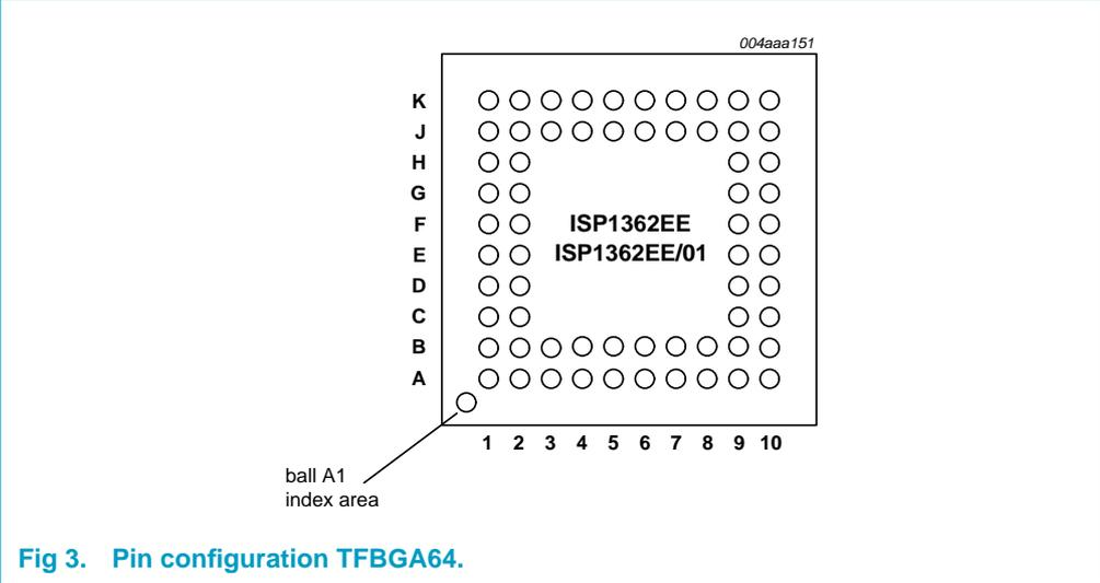
Fig 3. Pin configuration TFBGA64.
