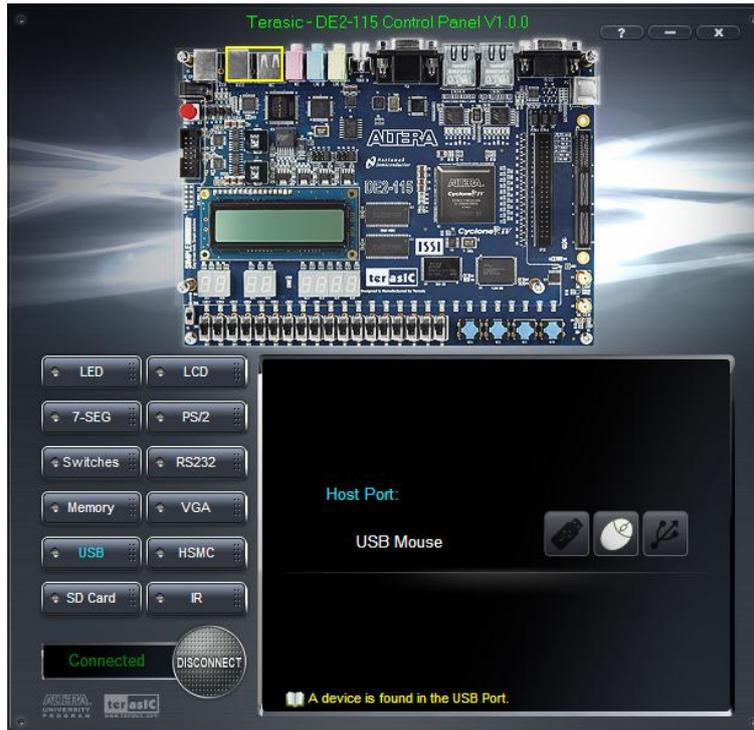
Figure 3-8 USB Mouse Monitoring Tool
