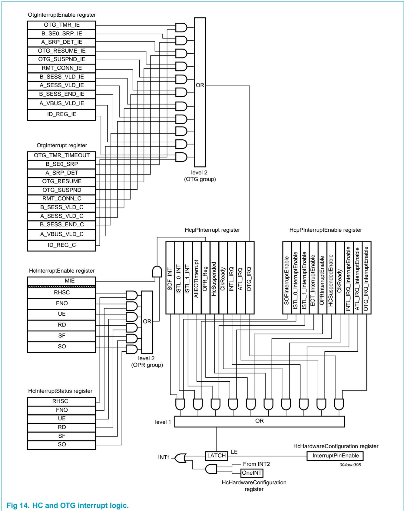
Fig 14. HC and OTG interrupt logic.
