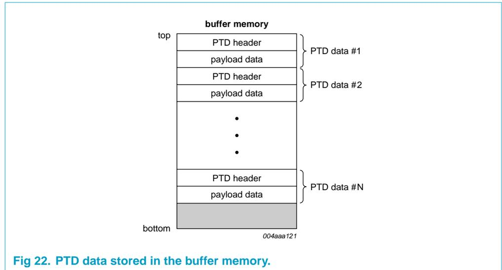
Fig 22. PTD data stored in the buffer memory.
