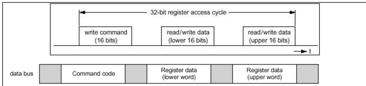
Figure 3-4: 32-Bit Register Access Cycle
