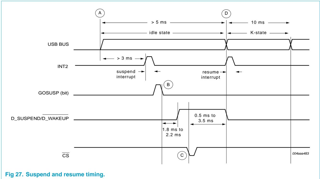
Fig 27. Suspend and resume timing.
