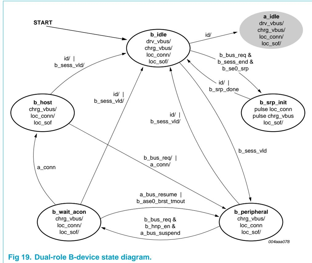
Fig 19. Dual-role B-device state diagram.
