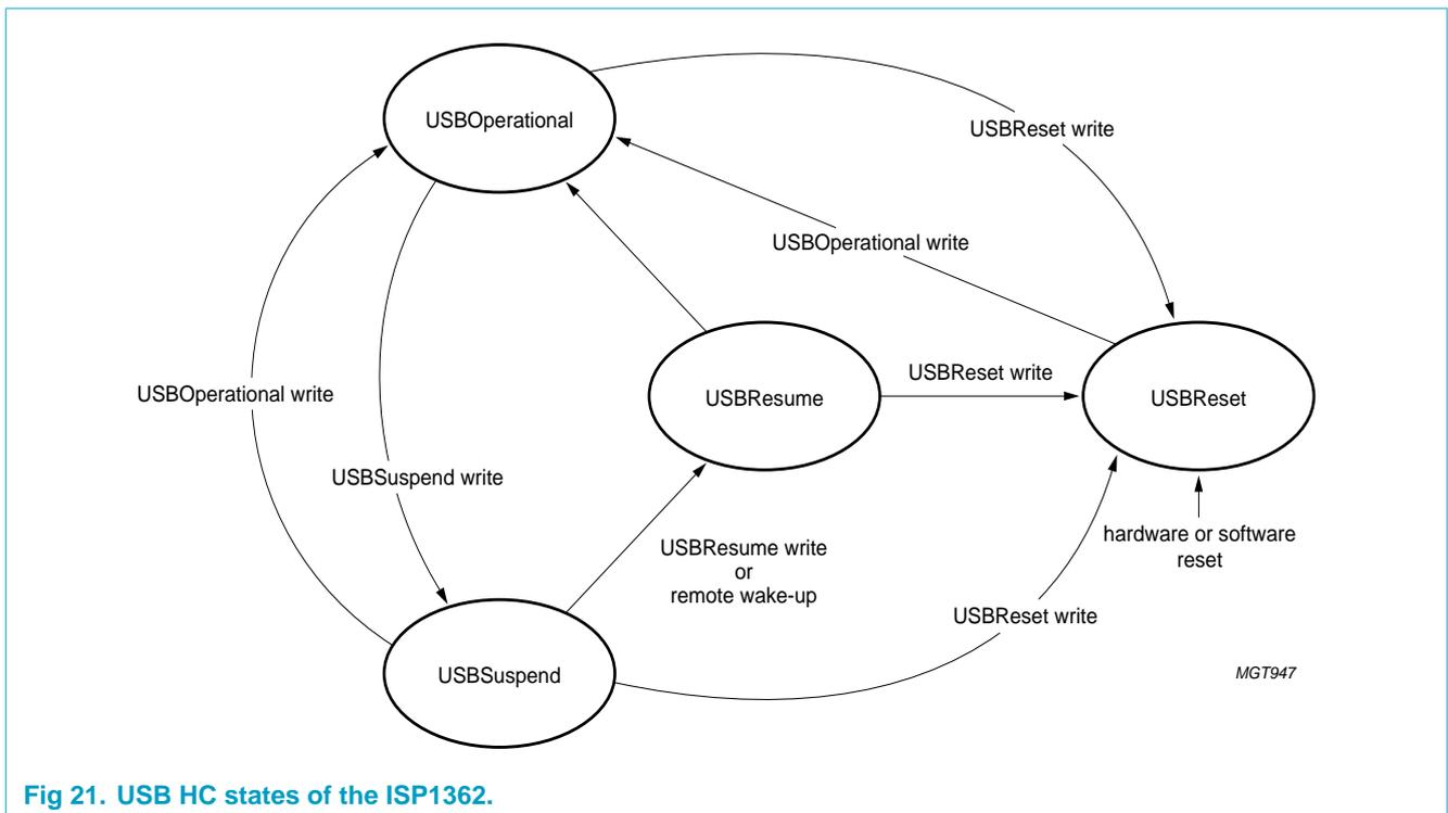
The USB states are reflected in the HostControllerFunctionalState (HCFS) field of the HcControl register. The HCD is allowed to perform only the USB state transitions shown in [Figure 21](#).
