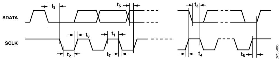
Figure 4. I<sup>2</sup>C Timing
