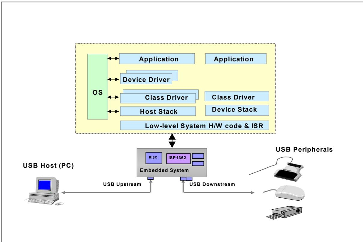
Figure 2-2: Software Model of the ISP1362
