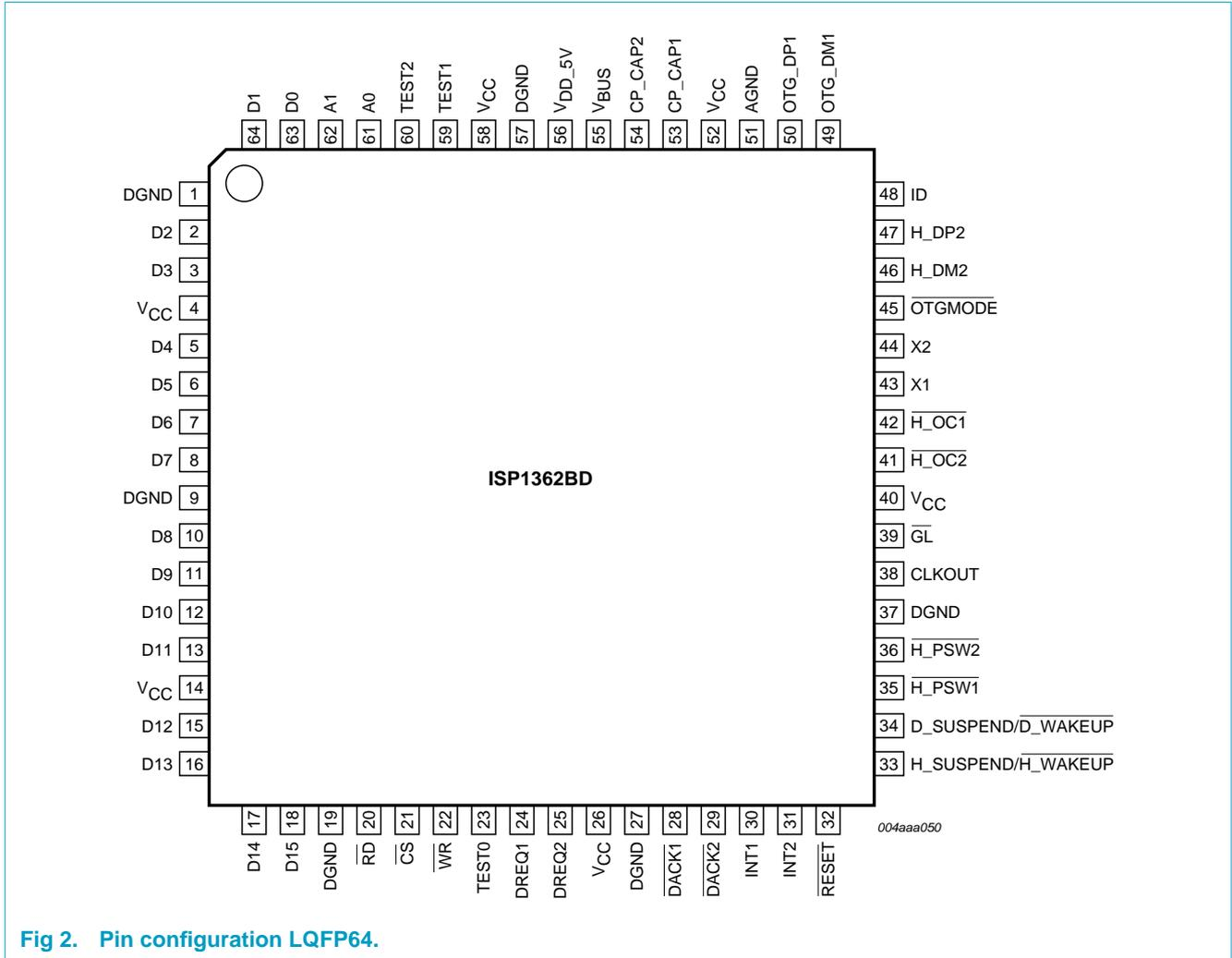
Fig 2. Pin configuration LQFP64.
