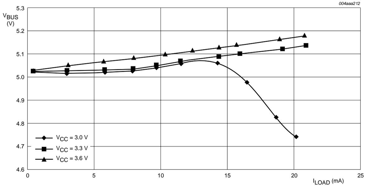
82 nF charge pump capacitor.
