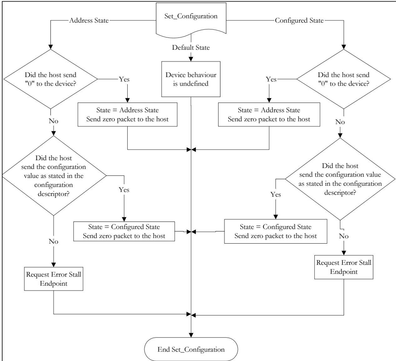
Figure 12-43: Flowchart of Set Configuration
