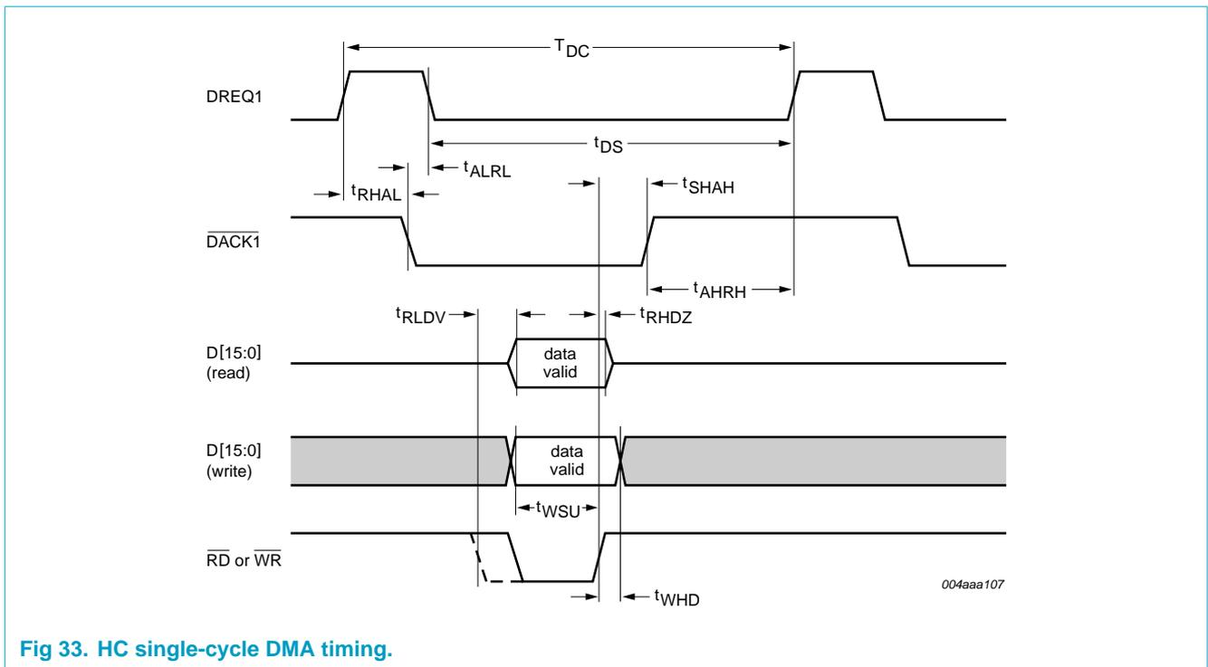
Fig 33. HC single-cycle DMA timing.
