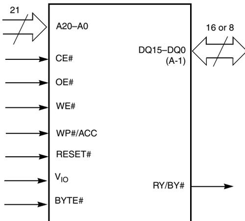
**Figure 5.5** S29GL032N Logic Symbol
