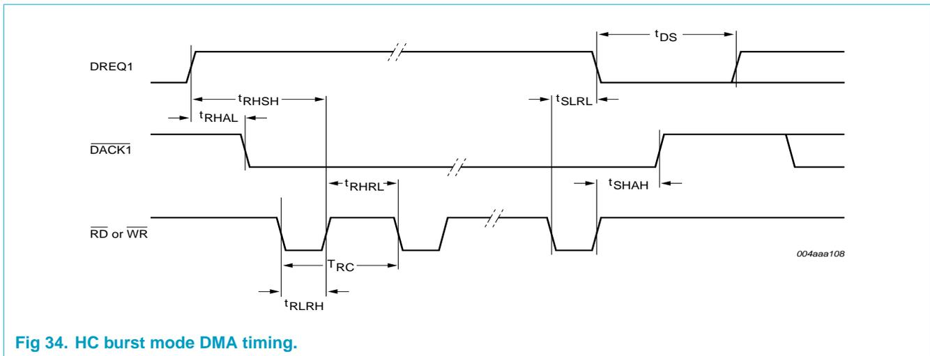
Fig 34. HC burst mode DMA timing.
