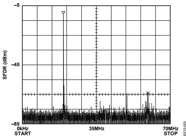
Figure 20. Single-Tone SFDR @  $f_{CLK} = 140$  MHz ( $f_{OUT} = 20$  MHz)
