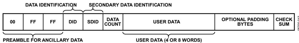
Figure 46. Gemstar- and CCAP-Embedded Data Packet (Generic)
