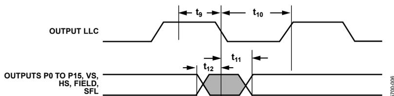
Figure 5. Pixel Port and Control Output Timing
