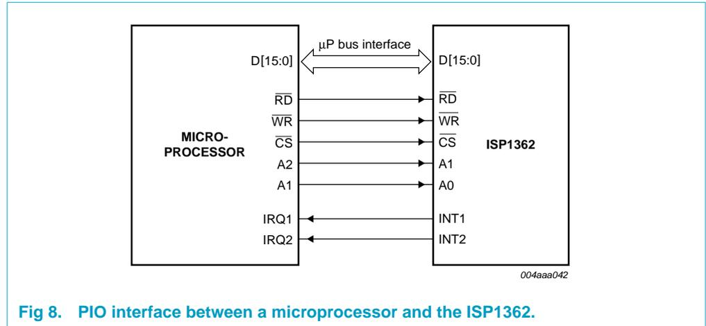
Fig 8. PIO interface between a microprocessor and the ISP1362.
