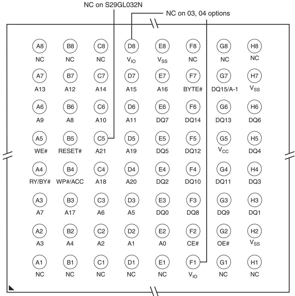
Figure 3.4 48-ball Fine-pitch BGA (VBK 048)
