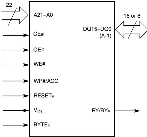
**Figure 5.2** S29GL064N Logic Symbol
