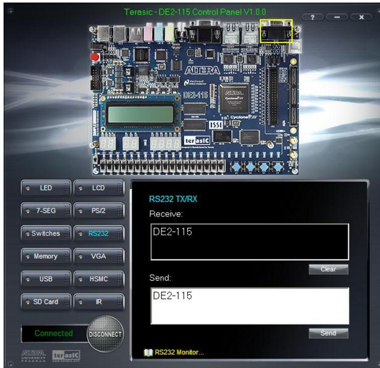
Figure 3-11 RS-232 Serial Communication
