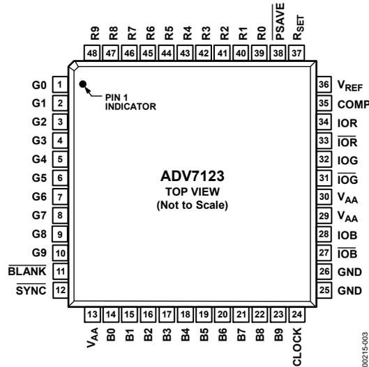
Figure 3. Pin Configuration
