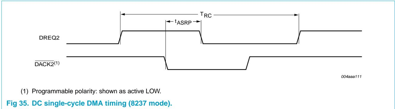
20.2.4 DC single-cycle DMA read timing in DACK-only mode
