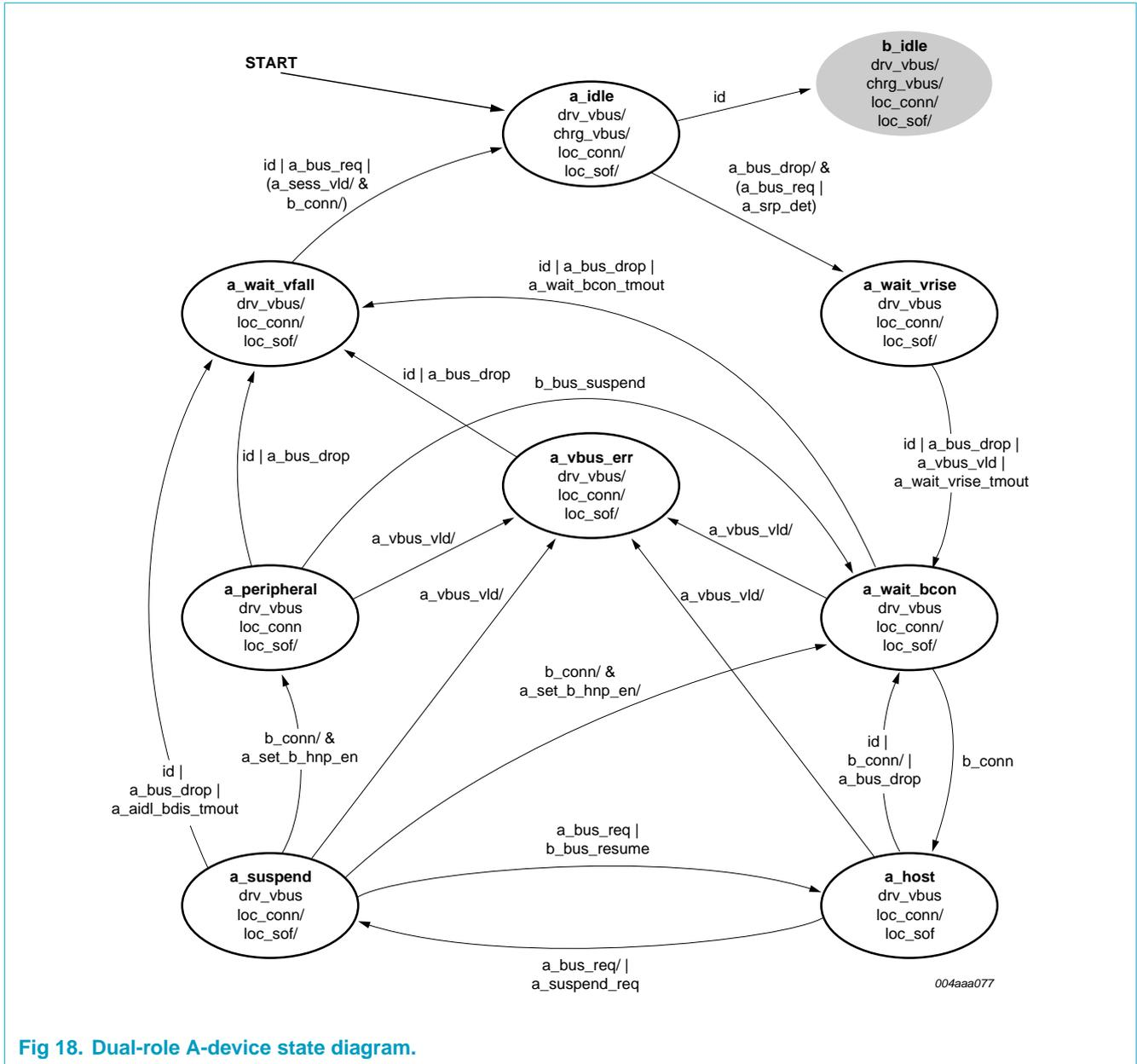
Fig 18. Dual-role A-device state diagram.
