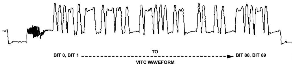
Figure 45. VITC Waveform and Decoded Data Correlation
