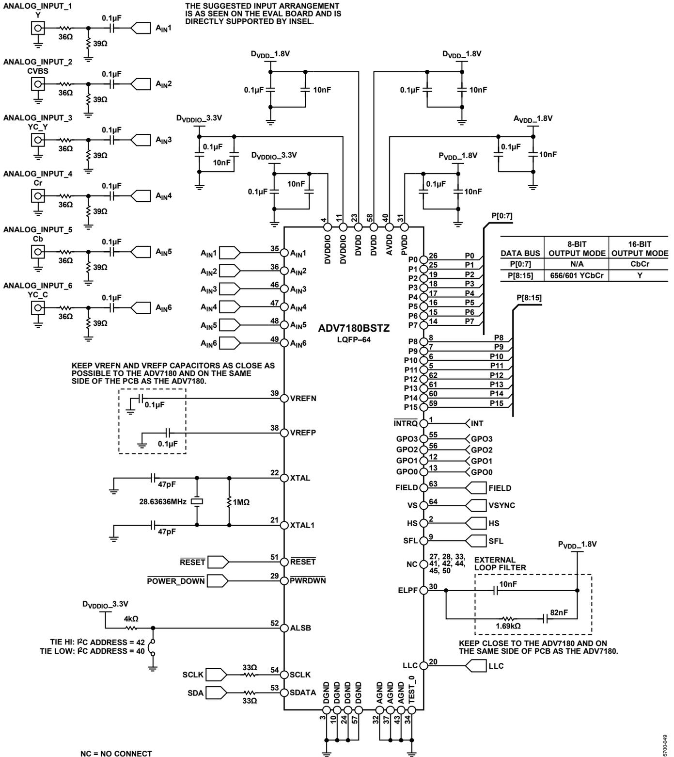
Figure 53. 64-Lead LQFP Typical Connection Diagram
