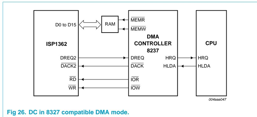
The following example shows the steps that occur in a typical DMA transfer:
