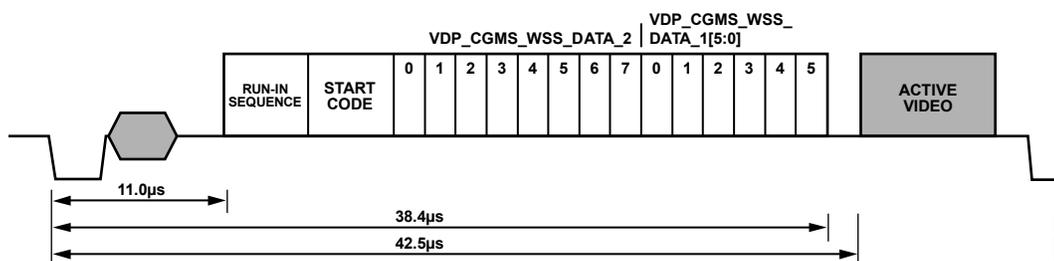
Figure 42. WSS Waveform
