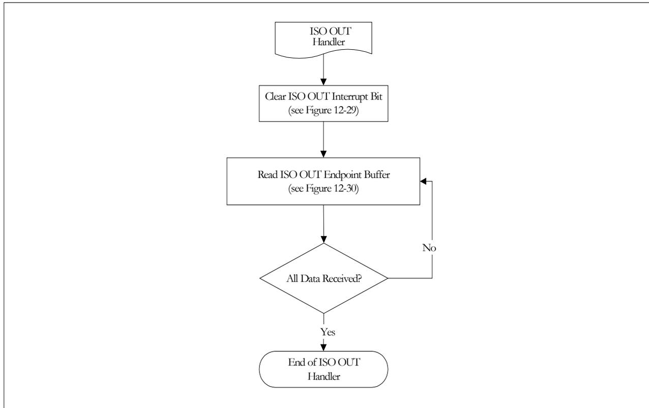
**Figure 12-27: Flowchart of the ISO OUT Handler**
