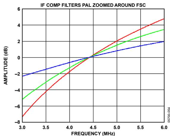
Figure 29. PAL IF Filter Compensation
