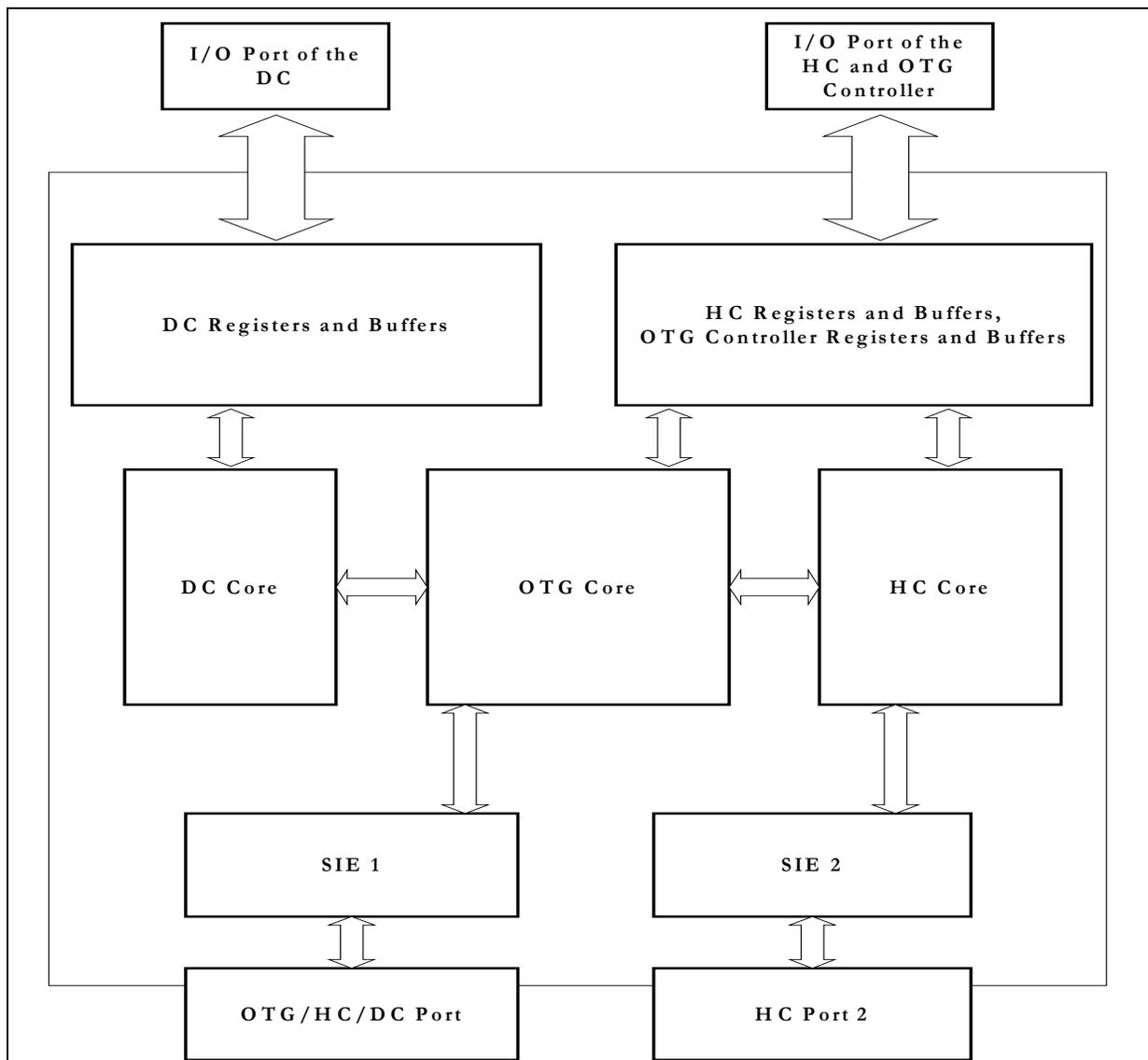
Figure 2-1: Programmer's Model of the ISP1362
