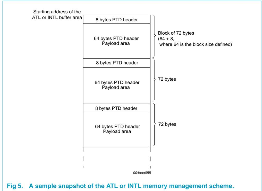
Figure 5 provides a snapshot of a sample ATL or INTL buffer area of 256 bytes with a block size of 64 bytes. The HCD may put a PTD with payload size of up to 64 bytes but not more. Depending on the ATL or INTL buffer size, up to 32 ATL blocks and 32 INTL blocks can be allocated. Note that a portion of the ATL or INTL buffer remains unused. This is allowed but can be avoided by choosing the appropriate ATL or INTL buffer size and block size.
