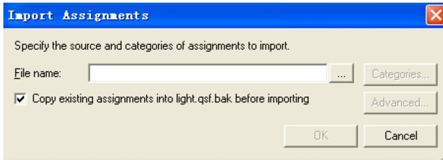
Figure 28. Importing the pin assignment.
