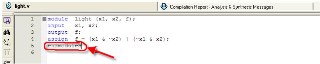
Figure 22. Identifying the location of the error.
