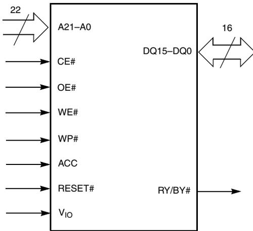
**Figure 5.4** S29GL032N Logic Symbol
