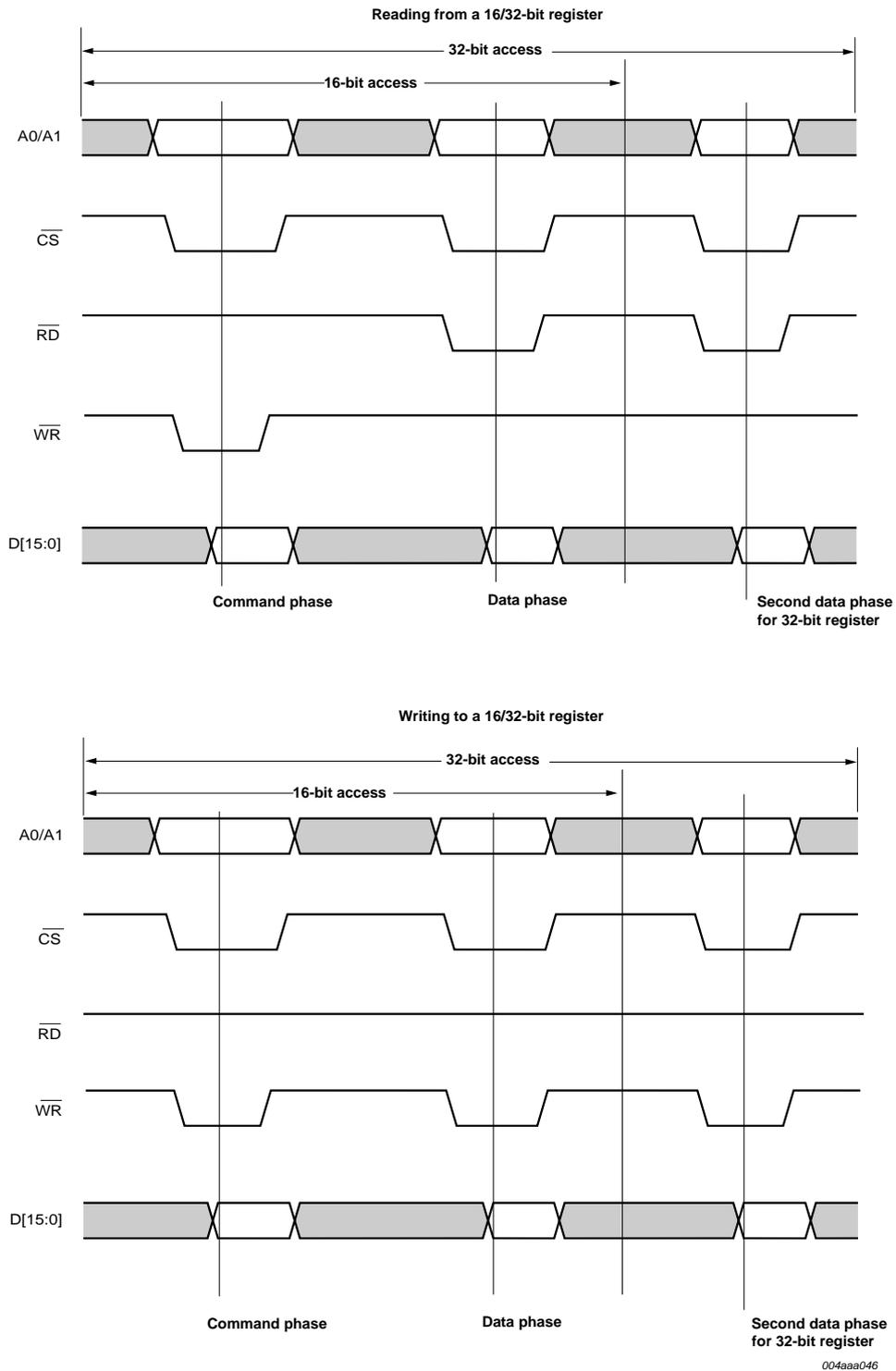
Fig 13. PIO access for a 16 or 32-bit register.
