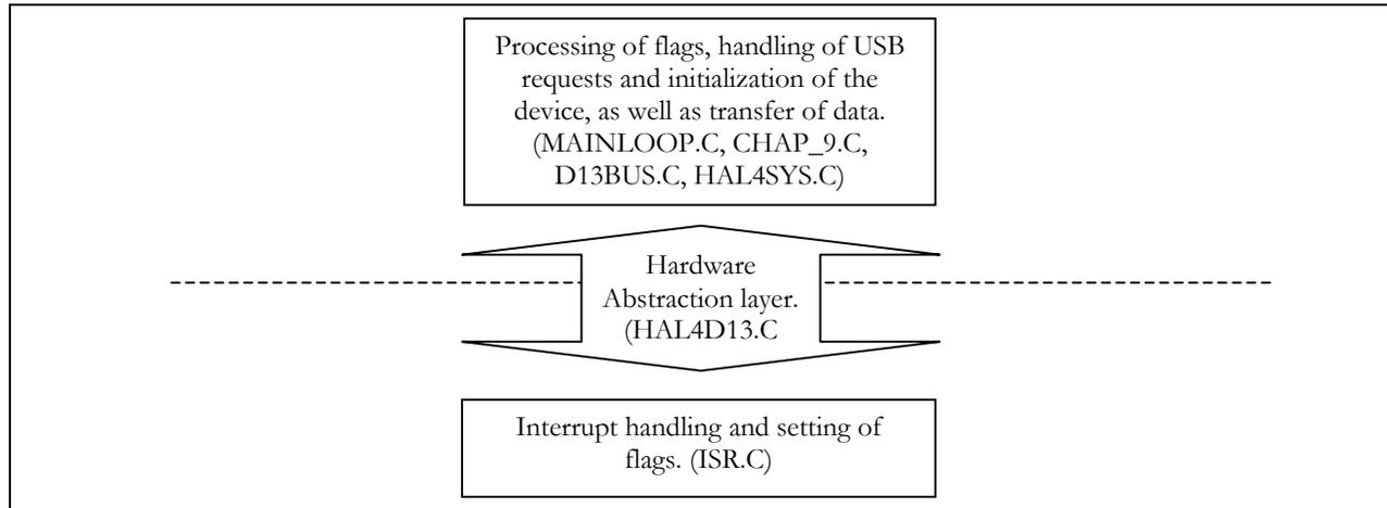
**Figure 12-1: Firmware Structure of the Device Controller of the ISP1362**
