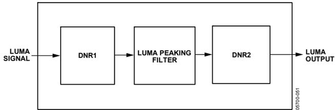
Figure 26. DNR and Peaking Block Diagram
