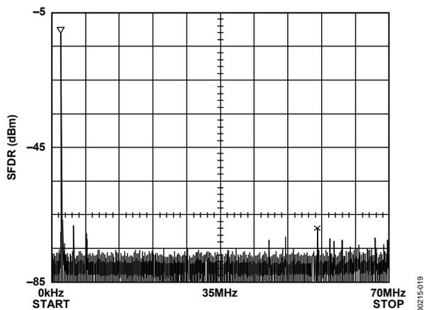
Figure 19. Single-Tone SFDR @  $f_{CLK} = 140$  MHz ( $f_{OUT} = 2$  MHz)
