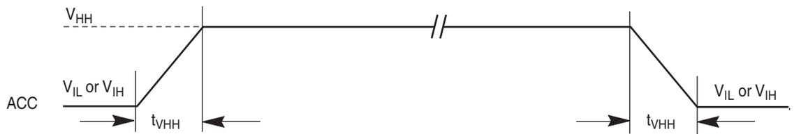
Figure 15.7 Chip/Sector Erase Operation Timings
