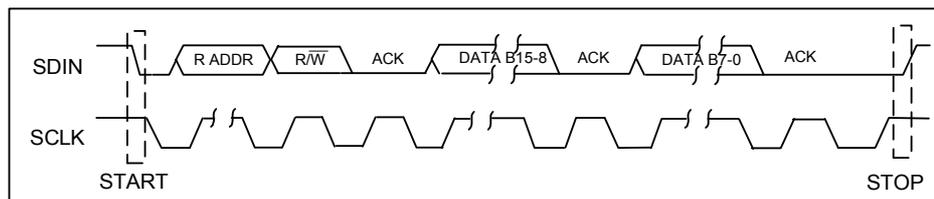
Figure 34 2-Wire Serial Interface
