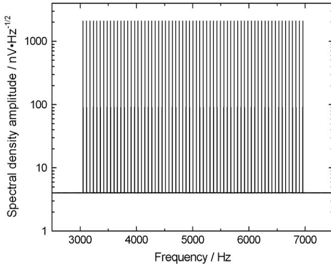
**Figure 3.** The calibration signal  $e_C$  for a bandwidth  $B = 3$  kHz to 7 kHz. The baseline is the Johnson noise  $e_N$ .
