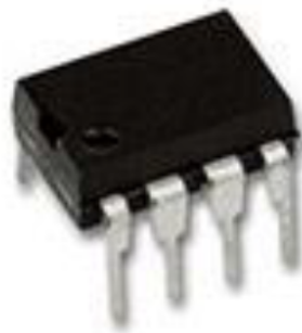
Dual-inline package (DIP) often used to package digital potentiometers
