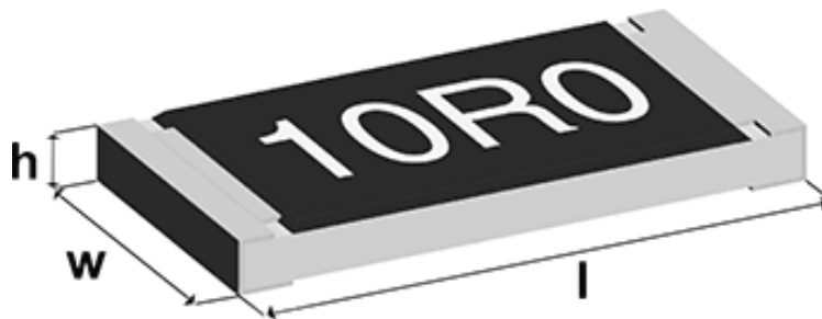
SMD resistor dimensions
