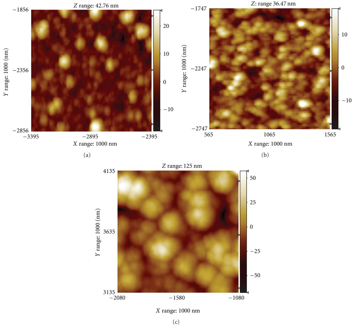
FIGURE 6: Noncontact atomic force microscopy (NC-AFM) images (topography) of films deposited by hot wire method at various process pressure. (a)  $P_p = 30$  mTorr (a-Si:H). (b)  $P_p = 90$  mTorr (onset of nanocrystallization). (c)  $P_p = 300$  mTorr (nc-Si:H).
