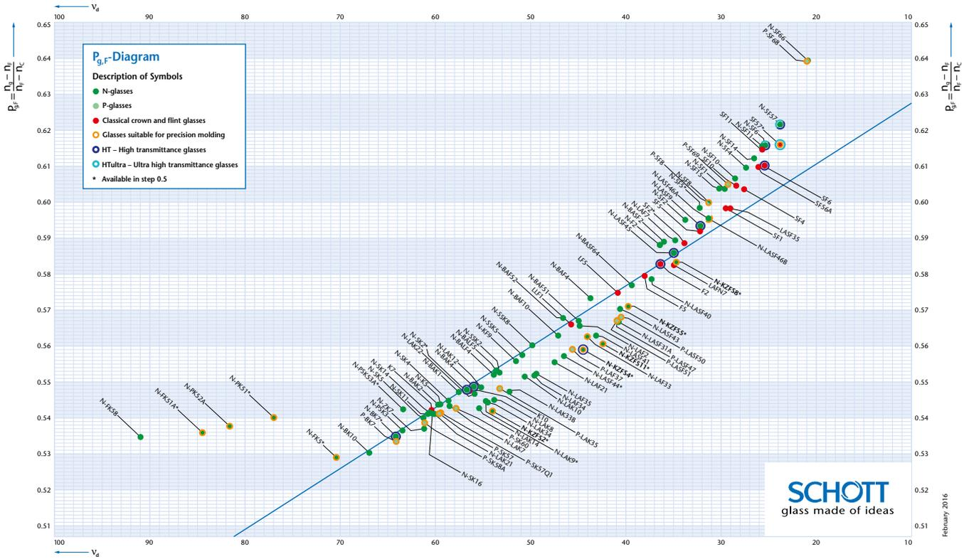
Fig. 2: P<sub>g,F</sub> as a function of the Abbe number for SCHOTT's optical glass assortment. Additionally the normal line is given.
