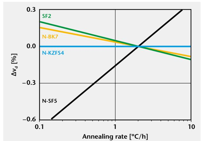
Fig. 4: Dependence of refractive index  $n_d$  (a: upper) and Abbe number  $v_d$  (b: lower) on the annealing rate for several glass types. Reference annealing rate is 2 °C/h [3].
