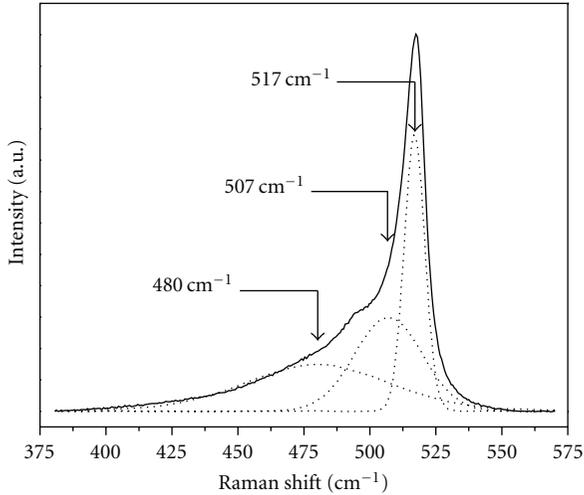
FIGURE 5: Deconvoluted Raman spectra for a nc-Si:H film prepared at  $P_p = 300$  mTorr with two Gaussian peaks and one Lorentzian peak and a quadratic base line, with an algorithm based on the Levenberg-Marquardt method [26].
