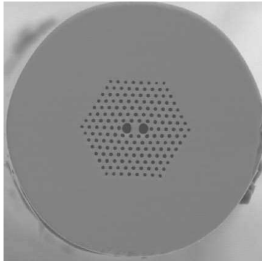
Figure 30 - SEM image of the highly birefringent MOF used for fabrication of the LPGs.
