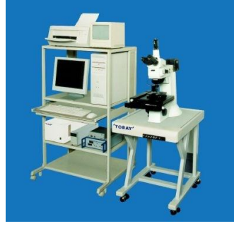
Figure 12. Surface profiler used for experiments.
