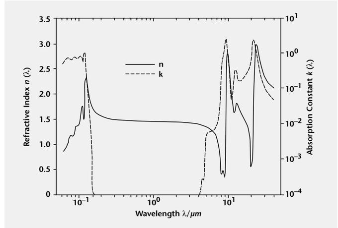
Fig. 1: Measured optical constants of fused silica (SiO<sub>2</sub> glass) [1].
