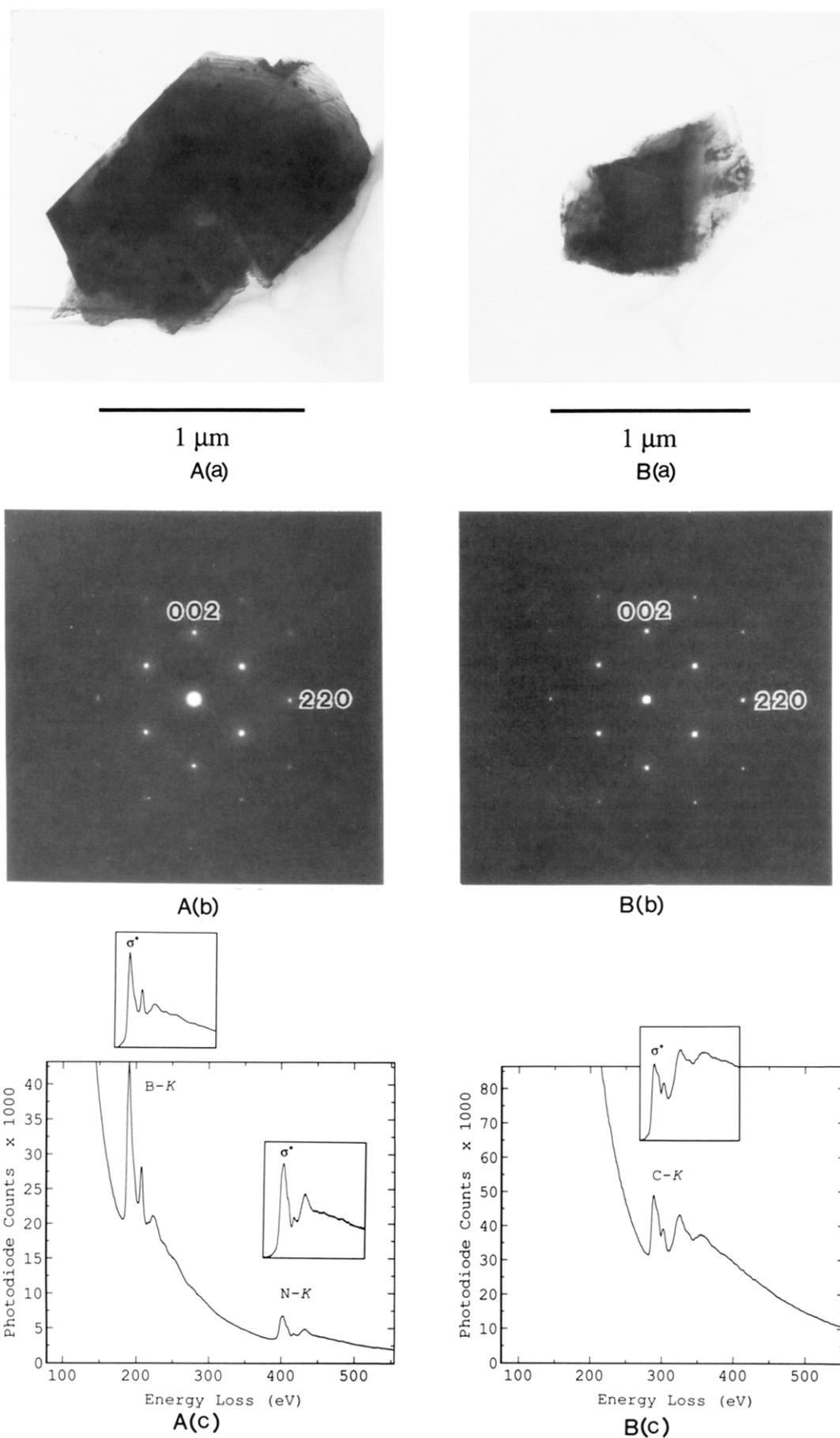
**Figure 3.** Two typical results of microanalyses on individual grains in the sample compressed at 5.5 GPa and 1500 °C. The labels A and B give (a) TEM image, (b) electron diffraction pattern of  $hhl^*$ , (c) K-edge electron energy-loss spectrum for the crystal fragments identified as cBN and diamond, respectively. The 002 and  $00\bar{2}$  spots in B(b) are to be absent according to the extinction rule.<sup>20</sup>
