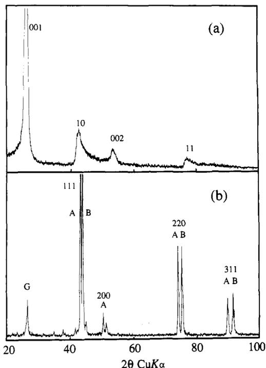
**Figure 2.** Powder XRD pattern for the graphitic  $BC_2N$  (a) before and (b) after the HP/HT treatment. Pressure 5.5 GPa; temperature 1500 °C; duration 20 min. The pattern in (a) is for the material deposited on a Ni metal chip at 850 °C and then annealed at 1800 °C under a  $N_2$  gas flow. The symbols A, B, and G denote two kinds of cubic phase and a graphitic residue, respectively.
