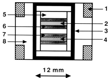
**Figure 4.** Sample assembly for the HP/HT treatments. 1, steel ring; 2, sample (ground  $\text{BC}_2\text{N}$ ); 3, graphite heater; 4, reference material (graphite powder or graphite + hBN); 5, 8,  $\text{NaCl} + \text{ZrO}_2$  (10 wt %) as a pressure medium; 6, 7, pressed disk of Co metal powder.
