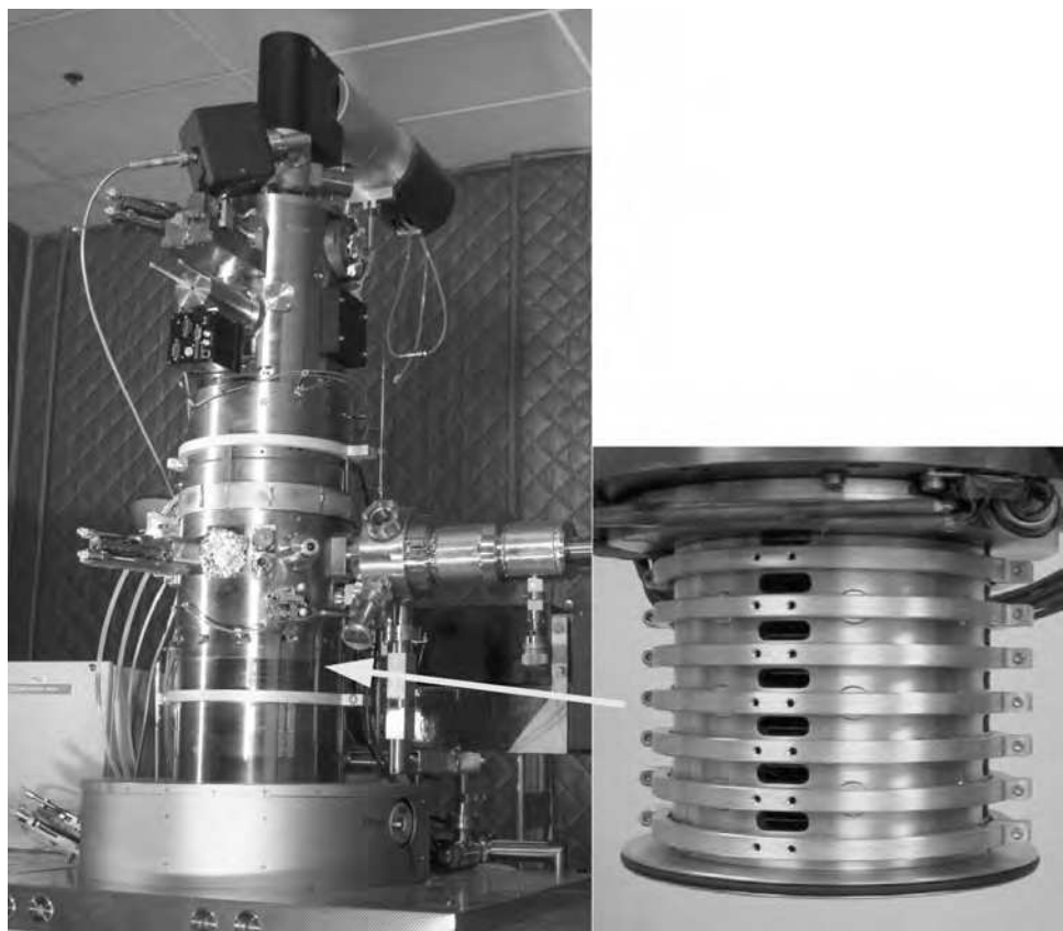
FIGURE 13.6 The 300 kV STEM at ORNL with aberration corrector (right inset).
