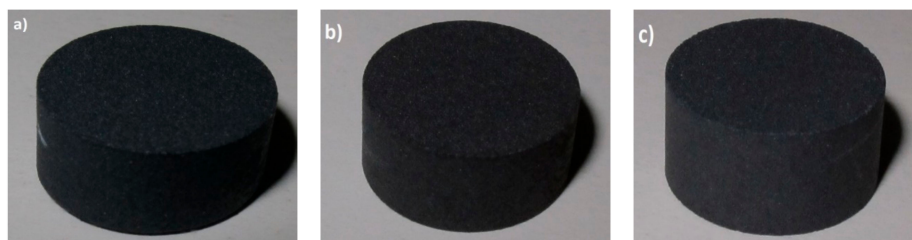
Figure 2. Photographs of the anodized Ti-15Mo discs treated in the electrolytes of series 9 (a), 10 (b), and 11 (c).
