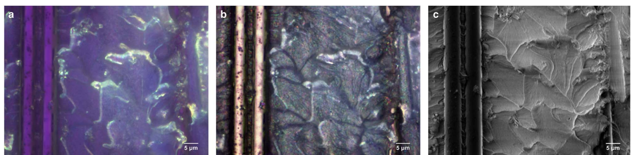
Figure 7. Images for 100× objective lens magnification. a: Light microscopic (LM) linear polarization; (b) LM bright field; (c) scanning electron microscope.
