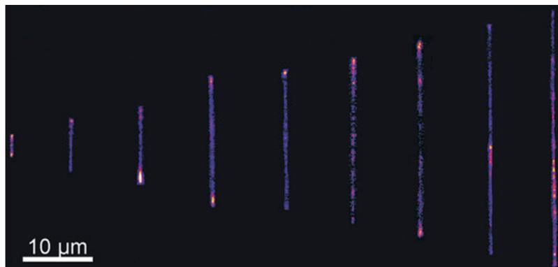
**Flow-Based Particle Trapping and Manipulation, Fig. 7** Time-lapse image of the relaxation dynamics of an individual single-stranded DNA molecule (ssDNA,  $L = 18 \mu\text{m}$ ) studied by the hydrodynamic trap based on a planar extensional flow. A single fluorescently labeled
