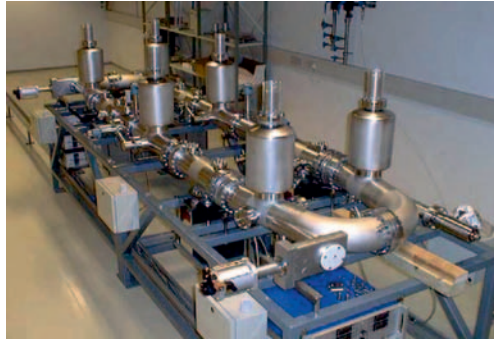
Fig. 1. Photo of compact electrostatic storage ring ELISA kindly presented by S. P. Moller [13]
