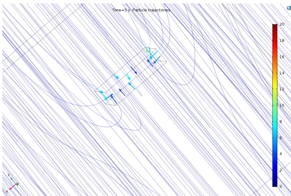
Fig 5. Closeup of some particle trajectory tracks, showing some that lead to wrap-around deposition on the bottom of the leaf.
