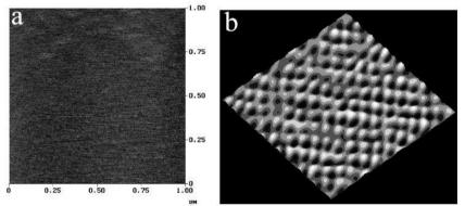
Fig.31 AFM images of ultra-flat  $TiO_2$  sample surface produced by a template stripping method after. (a) High resolution imaging of the  $TiO_2$  samples surfaces (b) shows atomic resolution of the  $TiO_2$  is frequently used in implants and the samples presented here are suitable to obtain molecular resolution of absorbed bimolecules with AFM.
