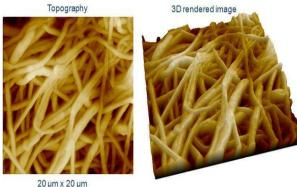
Fig.26: Applying of AFM at polymer nanofiber [53].
