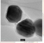
Fig.13: TEM micrograph of carbon nanocapsules encapsulating Co nanoparticle.
