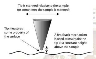
Fig.2: Basic principles of scanned probe techniques
