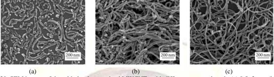
Fig. 20: SEM images of three kinds of as-received MWCNTs with different average length: (a)  $0.5\sim2~\mu\text{m}$ , (b) 30  $\mu\text{m}$ , and (c) 50  $\mu\text{m}$  [41].
