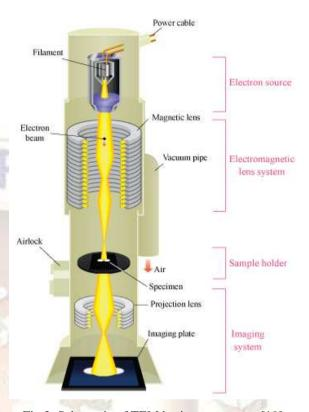
Fig.3: Schematic of TEM basic components [19]
