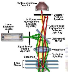
Fig.9: Schematic diagram of the optical pathway and principal components in a laser scanning confocal microscopy [33].
