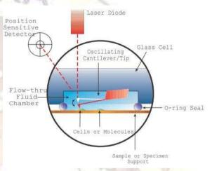
Fig.35: Fluid cell for an AFM which allows imaging in an enclosed, liquid environment [24].
