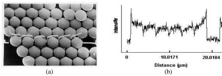
Fig.6: Intensity distance plot of a single row of spheres.
