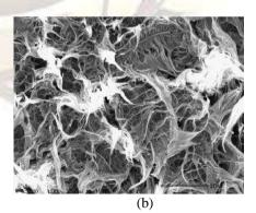
Fig.22: Fracture morphology of (a) UHMWPE/HDPE blend with ratio of 3:7 wt%. (b) UHMWPE/HDPE with 0.5wt% Carbon nanofiber [46].
