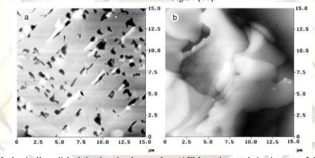
Fig.30: Mechanically polished titanium implant surface (AFM tapping mode in air z-rang 2.50µm) [48].
