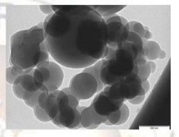
Fig.16: HR TEM image of nano-diamond particles manufactured by MW/RF method
