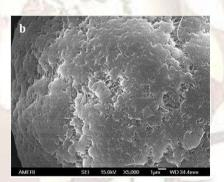
Fig.21: SEM micrographs of (a) UHMWPE Powder and (b) UHMWPE-CNT powder mixture.
