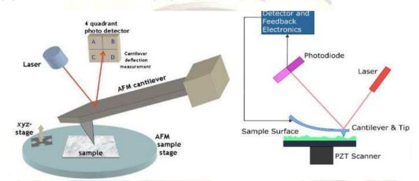
Fig.8: Operation of AFM surface analysis [6, 11, 12, 14]
