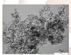
Fig.17: HR-TEM image of nanodiamond particles manufactured by detonation method.
