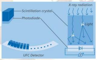
Fig.12: Sample of detector and how it operates.
