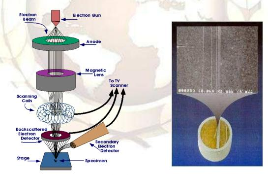
Fig.4: Schematic drawing of basic components of a typical SEM [26] Fig.5: Calibrate SRM 484f Sample [27]
