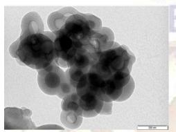
Fig.15: HR TEM image of manufactured nanodiamond particles by microwave/radiofrequency (MW/RF) method
