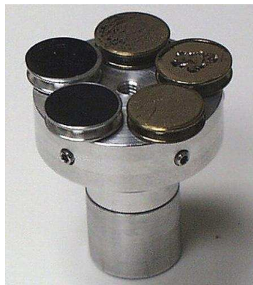
Fig 13.SEM sample holder
