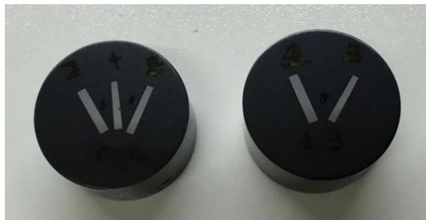
Figure 4.23 Samples mounted with PolyFast powder.
