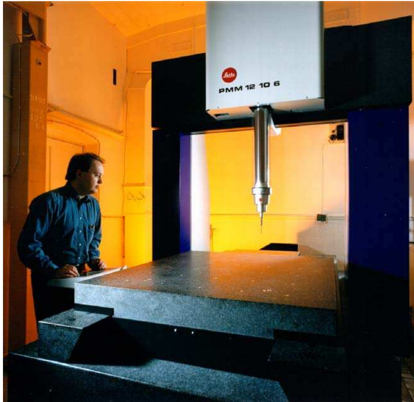
Figure 26 A typical bridge type CMM
