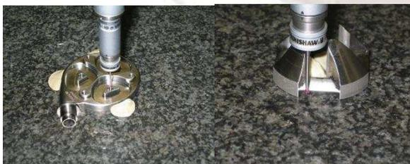
Fig.43: Inspection of artificial heart pump using CMM [60]
