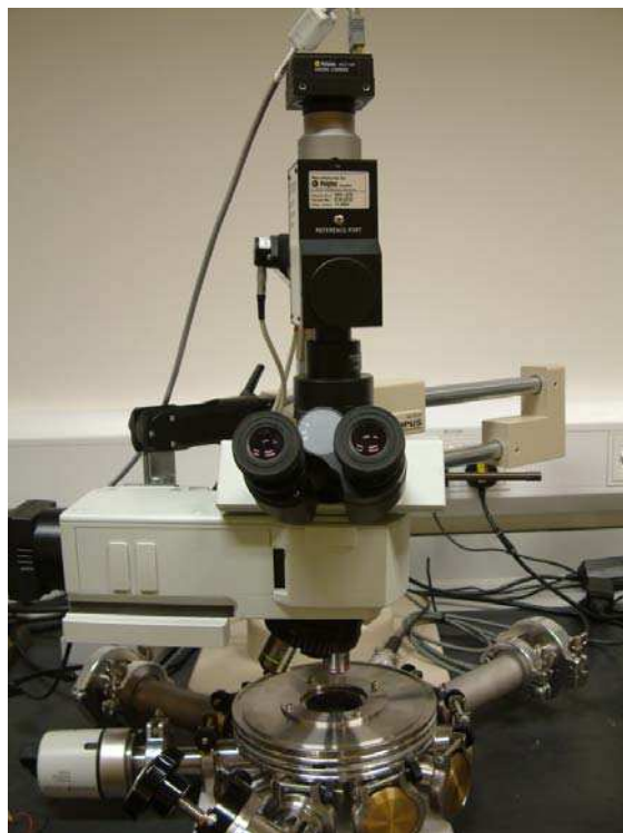
Figure 30 Photograph of the vibrometer system in use at NPL. The scanning LDV unit is positioned on top of the microscope, with the vacuum chamber beneath the microscope objective lens
