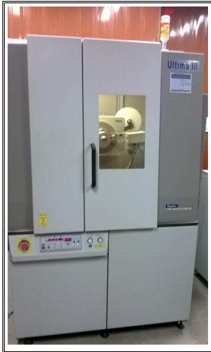
Figure 3.5 : Photograph of Rigaku Ultima III X-ray Diffractometer
