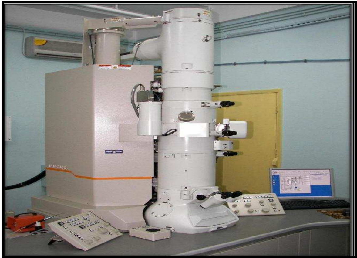
Figure 3.4 : HRTEM (JEOL 200 kV) SET UP
