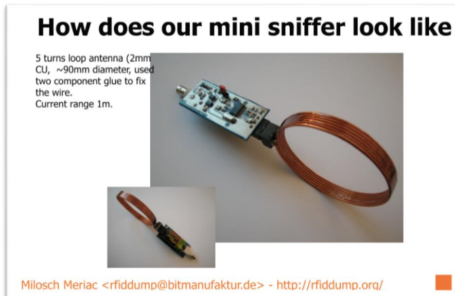
Figure 3-1 Long range custom RFID reader design
