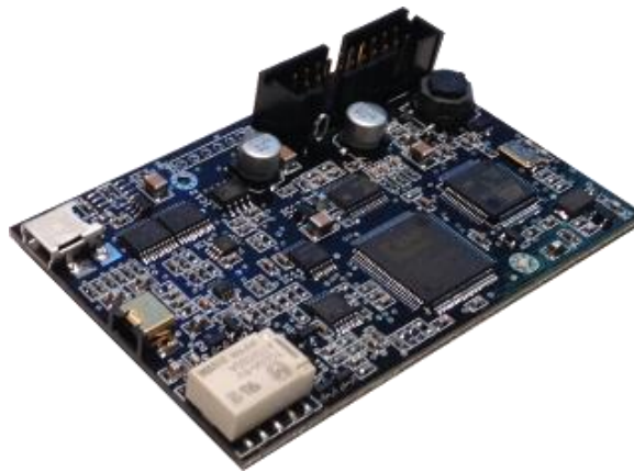
Figure 7-1 Proxmark III device
