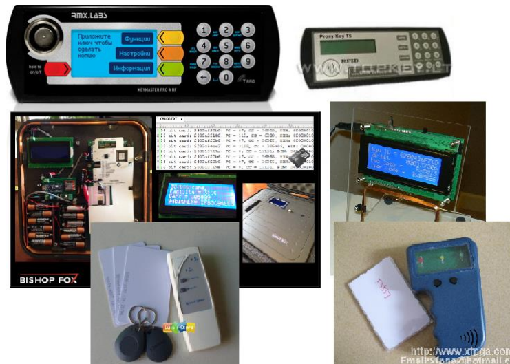
Figure 3-5 Automated RFID tag cloner devices
