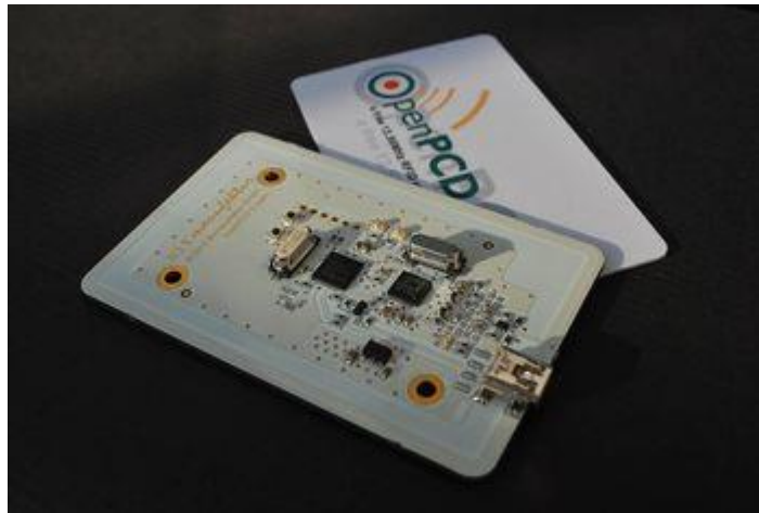
Figure 7-2 OpenPCD 2 design, a 13.56MHz RFID & NFC reader and emulator
