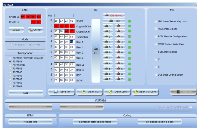
Figure 4.4: We use the commercial MiraClone tool to read the remote secret key and edit the counter pages in the transponder EEPROM.
