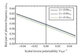
FIG. 2. Mapping between plasmon frequency  $\omega$  and the eigenvalue  $\alpha^{-1}$  for Drude model of different damping coefficient  $1/\tau$  (see Eq. 5). The mapping is nearly linear in the range of interested shown in Fig. 1 (b) (i.e.,  $0.64\omega_p > \omega > 0.50\omega_p$ ). The real part decreases when one increases the damping coefficient.
