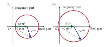
FIG. 3. Representation of  $(d-t)^3 + t^3 \exp(-ikd)$  in complex plane. The complex number evolves as kd changes from  $-\pi$  to  $\pi$  for (a) t < d/2 and (b) t > d/2. In (b), winding number is non-zero, which leads to non-zero Zak phase.
