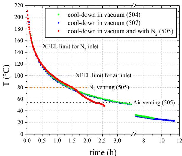
Figure 10: Measurement done during the cool-down of DCV cavities after the completion of the equatorial welding operation. Cool-down in vacuum (blue and green curve); Cool-down in vacuum and then N<sub>2</sub> venting (red curve).
