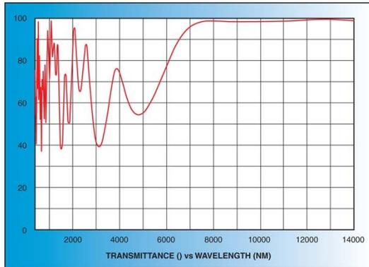
Figure 1: ZnSe viewport transmittance vs wavelength [6].
