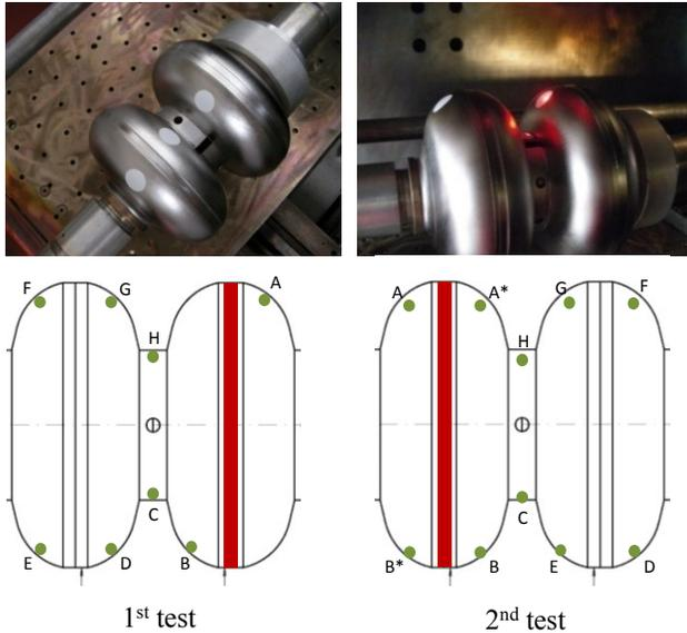
Figure 4: Up: photos of the two-cell dummy cavity before and during tests. Red laser beams are used for aligning the pyrometer on the dots. Down: positions of the “emissive dots” in the two tests configuration.
