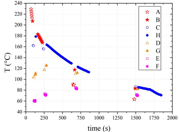
Figure 5: Temperature at different locations of the two-cell cavity (1<sup>st</sup> test). For dot positions see Fig. 4.
