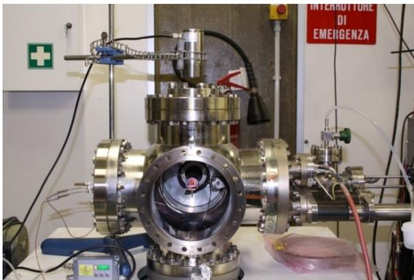
Figure 2: Set up at LASA with pyrometer mounted on top of the test chamber.
