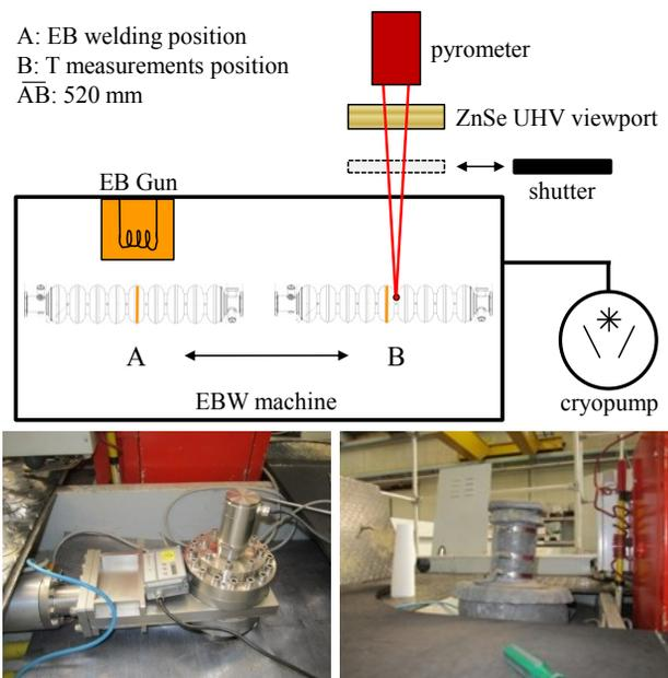
Figure 3: Sketch of the experimental setup and photo of the pyrometer mounted on a gate valve with and without X-ray shielding.
