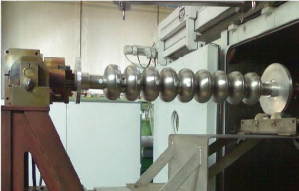
Figure 7: The 1.3 GHz 9-cell dummy cavities used for the infrared pyrometer temperature measurements. The “emissive dots” are placed not only close to the equators but also on the beam pipe tube and on the stiffening rings.
