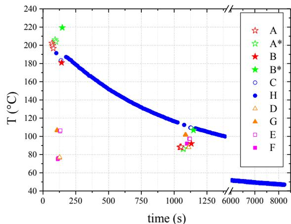
Figure 6: Temperature at different locations of the two-cell cavity (2<sup>nd</sup> test). For dot positions see Fig. 4.
