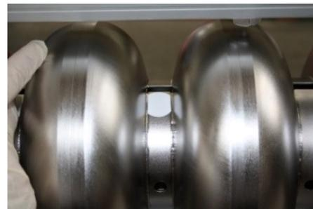
Figure 9: DCV under preparation for the equatorial welding. One “emissive dot” is used to read the stiffening temperature during welding operation.
