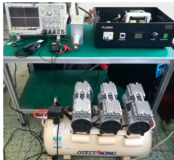
Figure 19. Experimental platform of resonant power supply system for plasma cleaning.
