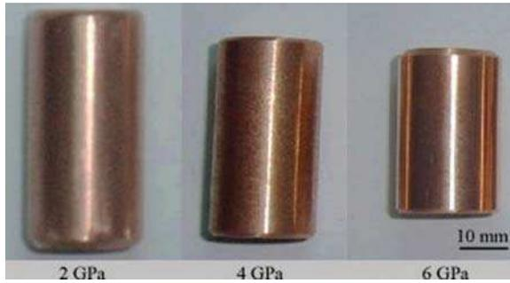
**FIGURE 5.3** Cu/ $\alpha$ -Al<sub>2</sub>O<sub>3</sub> bulk sample under three levels of explosion pressure [34]. (Reprinted with permission from Zhao Z, Li X-J, Tao G. Manufacturing nano-alumina particle-reinforced copper alloy by explosive compaction. *J Alloys Compd* 2009;478:237–239, Copyright 2009, Elsevier.)
