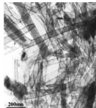
Figure 18. \text{SnS}_2 nanotubes sample synthesized with hydrothermal method. Reprinted with permission from ref 169 (Figure 3c). Copyright 2003 Springer.
