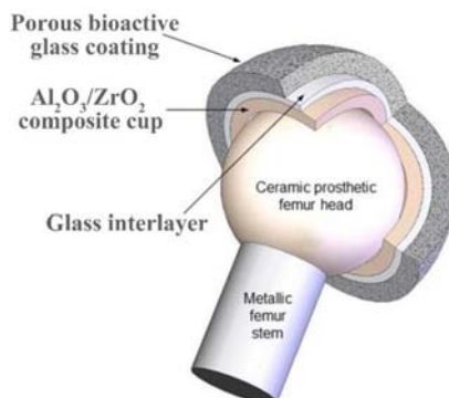
Figure 6.5 Usage of Al 2 O 3 –ZrO 2 composites in hip prosthesis [3].
