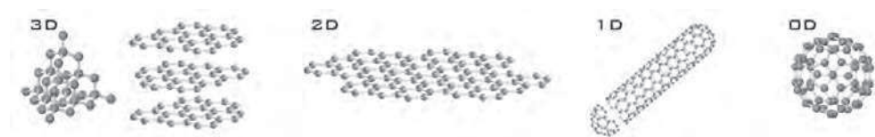
Fig. 1. Crystal structures of different allotropes of carbon. (Left to right) Three-dimensional diamond and graphite (3D); two-dimensional graphene (2D); one-dimensional nanotubes (1D); and zero-dimensional buckyballs (0D) (Mikhail & Katsnelson, 2007).
