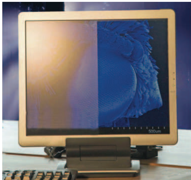
Figure 22 (online color at: www.lpr-journal.org ) Photo taken from a flat-panel display with standard antiglare surface (left side) and combined 'moth-eye' anti-reflective and antiglare surface (right side). As an object on the flat-panel display the compound eye of a moth is shown (courtesy of Volkmar Boerner; Holotools, Freiburg).
