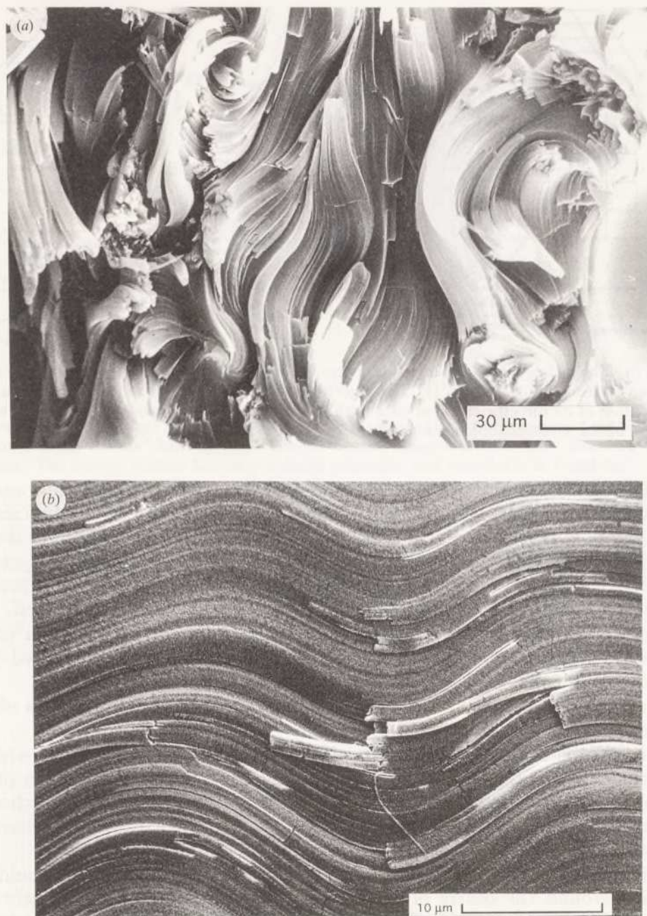
Figure 1. (a) Fracture surface revealing the local director orientation in a sample which would show a schlieren texture in transmitted polarized light. Material: random copolymer of 75% hydroxybenzoic acid and 25% hydroxynaphthoic acid. M_W = 5800 . Courtesy, Dr A. Anwer. (b) Fracture surface through a thin sample of the same polymer as in (a). It has been sheared and quenched and shows a banded texture in transmitted polarized light. The fracture plane is parallel to the shear plane and the shear direction is horizontal. Courtesy, Dr T. J. Lemmon.
