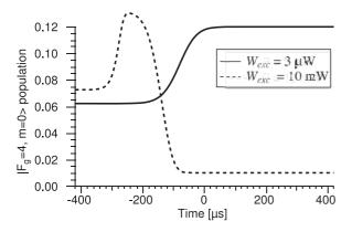
FIG. 10. Evolution of the  $|F_g=4,m=0\rangle$  state population during the atom propagation across the excitation laser beam resonant with the T44 transition. The quite different behaviors for low and high radiation powers, expected to correspond to regimes (ii) and (iii), are shown with solid and dashed lines, respectively.
