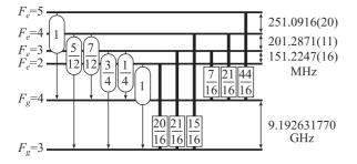
FIG. 5. Branching ratios  $\Pi_{F_a,F_b}$  (arrows with rounded frames) for  $6^2S_{1/2} \rightarrow 6^2P_{3/2}$  HF transitions and relative line strengths  $\tilde{S}_{F_aF_b}$  (thick lines with rectangular frames). HF frequency splittings are also shown [31].
