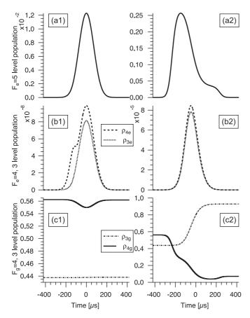
FIG. 7. Evolution of the populations in the hyperfine sublevels (a1), (a2)  $F_e$  = 5, (b1), (b2)  $F_e$  = 3, 4, and (c1), (c2)  $F_g$  = 3, 4 during the atom propagation across the excitation laser beam resonant with the T45 transition. Laser power is  $W_{exc}$  = 3  $\mu$ W (corresponding to  $I_{exc}$  = 58  $\mu$ W/cm<sup>2</sup>) in (a1), (b1), and (c1) and  $W_{exc}$  = 10 mW (corresponding to  $I_{exc}$  = 190 mW/cm<sup>2</sup>) in (a2), (b2), and (c2).
