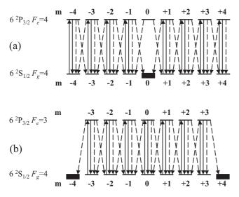
FIG. 2. Zeeman structure for the (a) T44 and (b) T43 transitions upon  $\pi$  polarized excitation. The solid arrows show the absorption and stimulated emission transitions, while the dashed ones depict the spontaneous emission paths. The thick levels denote the population accumulation due to optical pumping.
