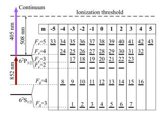
FIG. 1. (Color online) Excitation and photoionization scheme for cesium  $D_2$  line with hyperfine structure and magnetic Zeeman sublevels. Laser excitation occurs from  $F_g = 4$ . Magnetic Zeeman sublevels are numbered according to Eqs. (13).
