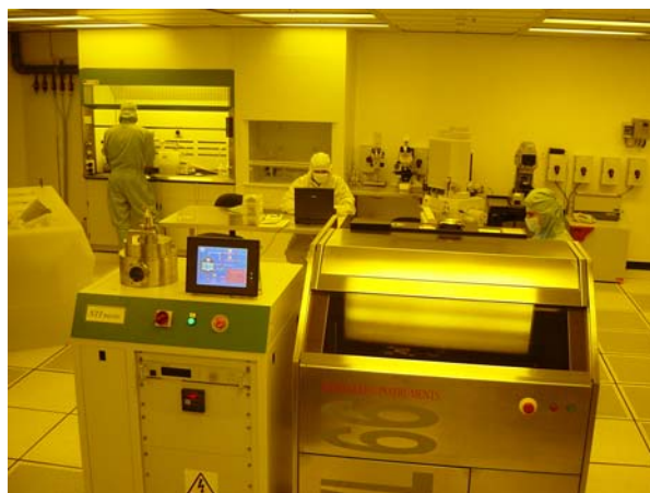
Fig. 3: View of the clean room. Laser direct writer and plasma cleaner in the foreground, behind the scanning electron microscope with electron beam lithography add on. In the background from left the electroplating wet bench, chemical hoods, and the optical metrology.
