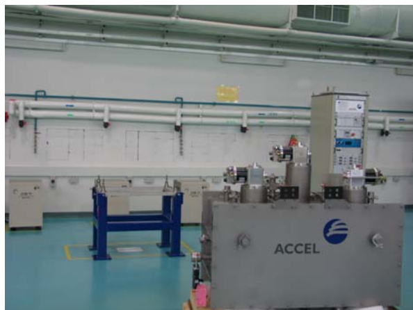
Fig. 14: Supramini vessel, girder, 3 cryocoolers, and power supplies and controls.
