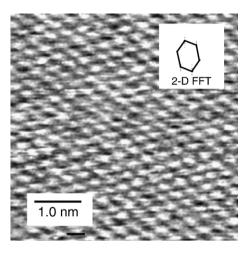
Fig. 2. STM image (scan size  $5.0 \times 5.0$  nm) of a fresh, unexposed HOPG surface; raw data are shown. In the inset: 2-D FFT map of the STM image; peaks are located at the vertices of a hexagon, in agreement with the graphite lattice structure (lines connecting data points are guides to the eye).
