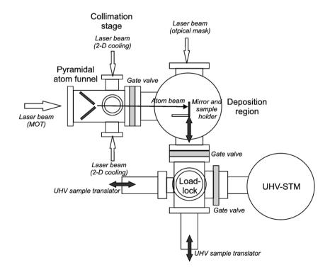
Fig. 1. Sketch of the experimental apparatus; the whole system consists of a set of interconnected UHV chambers separated by gate valves and evacuated by ion pumps (base pressure below  $10^{-9}$  mbar), except the load-lock region, which is pumped by turbo dry pumps. Magnetic translators are used to transfer the sample from the deposition to the investigation (STM) region.
