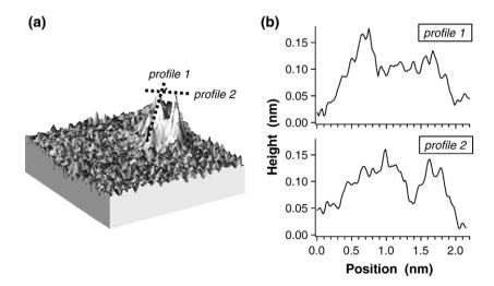
Fig. 3. 3-D view of an STM image acquired on an HOPG surface exposed to the laser cooled cesium beam (scan size  $6.0 \times 6.0$  nm); cesium structures are clearly visible, superimposed to the ripples representing the graphite lattice structure (a); line profile analyses along the two directions marked by dotted lines in the left panel (b).
