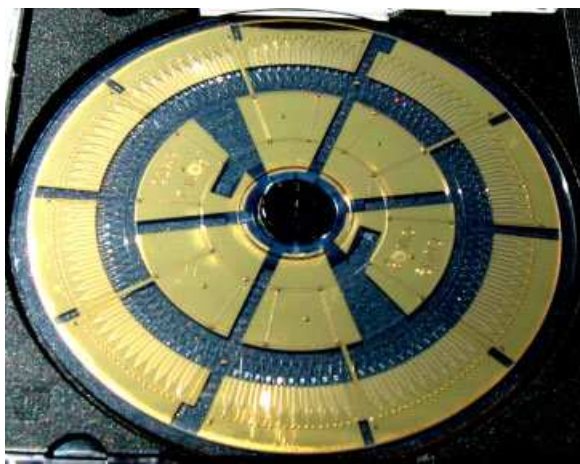
FIGURE 7. Photograph of a centrifugal CD for high-throughput MALDI-MS from a chip. [Color figure can be viewed in the online issue, which is available at www.interscience.wiley.com .]
