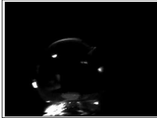
Figure 3.80 Picture of a meniscus before electrical activation. The wetting front of the meniscus is well defined and thus no wetting of the emitter lateral surfaces takes place.
