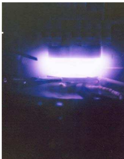
Figure 5. Photograph of D. C. sputtering plasma.
