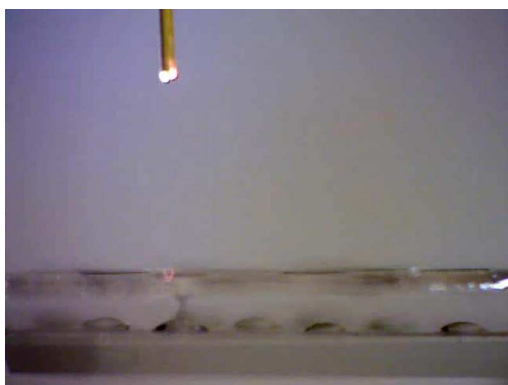
FIG. 5. Serial dispenser from nine almond oil droplets (about 1 \mu\text{l} each). Reservoir drops from the bottom are stimulated selectively and sequentially one at the time by the laser beam incident on the single GNR disk-film on the front of the matrix. The distance between the two glass slides is 2 mm and the size of the optical fibre is 300 \mu\text{m} . In the movie it is possible to see that droplets in the middle and rear rows behaves in the same way thus yielding a serial dispenser which may be addressed with a fibre tip (enhanced online) [URL: http://dx.doi.org/10.1063/1.4825337.2 ].
