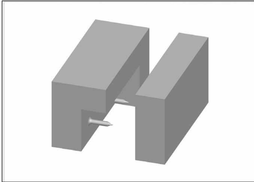
Figure 4.8 Schematic of a pencil matrix section where the fuel container edge is present. Appropriate periodicity boundary conditions were taken to make the finite element results useful for the comparison of edge influence in the electric field surrounding the emitters.
