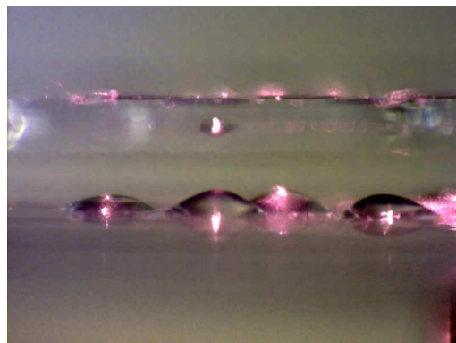
FIG. 4. Side view of a multi dispenser of five almond oil droplets (about 1 \mu\text{l} each). These drops are positioned on the lower glass slide right below the GNR films placed onto LN wafer. The distance between the two glass slides is 2 mm. Laser radiation lights an area of 1.5 cm diameter, so that the films are simultaneously illuminated from above. In the movie it is possible to see a sequence of liquid shootings where the almond oil drops dispense small droplets onto the above glass slide (enhanced online) [URL: http://dx.doi.org/10.1063/1.4825337.1 ].
