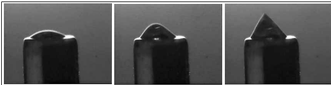
Figure 1.5 Sequence that illustrates the transition of an spherical meniscus into a Taylor Cone.
