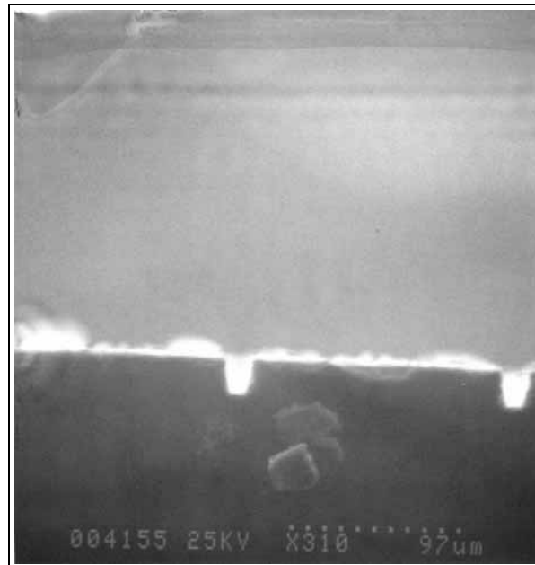
Figure 3.53 SEM picture of a test wafer with a channel formation 25\ \mu\text{m} deep, showing the same cross-sectional parametrization of Figure 3.52. The ruler that appears on the picture is 1.1 - 1.2 times larger than in reality (a way to tune the ruler is check the 130\ \mu\text{m} channel separation).
