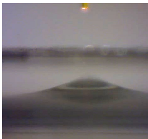
FIG. 7. Droplet dispensing from a large reservoir. The GNR-LN comprises a single 10 mm large GNR film placed onto a LN crystal. The GNR-LN device is stimulated locally by laser light escaping from the tip of an optical fibre. Due to the pyro-electrohydrodynamic force the surface of the liquid reservoir has changed to exhibit a conical tip. The distance between the water surface (when it is not undergoing the electric field) and the upper glass slides is 2 mm and the size of the optical fibre is 300 \mu\text{m} . In the movie the fibre position is moved through different sites (enhanced online) [URL: http://dx.doi.org/10.1063/1.4825337.3 ].
