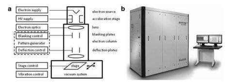
**Fig. 2.2** Electron beam exposures systems: (a) schematic diagram, (b) Raith 150<sup>TWO</sup> commercial EBL system (used with permission [7])
