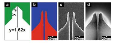
**Fig. 2.27** (a) Diagram of an alternative clamping point design with an optimized side width of x = 165 nm, (b) the final dissolution profile compared with (c) a SEM image of the developed PMMA resist, and (d) a SEM image of the released SiCN resonator clamping point [53]
