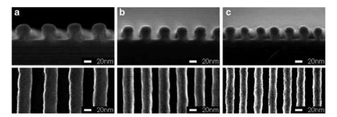
**Fig. 2.14** Cross-section and top-view SEM micrographs showing examples of optimized dense nanoscale gratings fabricated in PMMA using a Raith 150 system with 10 keV voltage, and employing various development temperatures: (a) RT, 70 nm pitch; (b)  $-10^{\circ}$ C, 50 nm pitch; and (c)  $-15^{\circ}$ C, 40 nm pitch [29]
