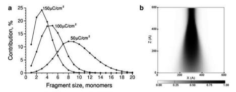
**Fig. 2.6** (a) Calculated distribution of PMMA fragment sizes for various doses at 10 keV [26]. (b) Spatial distribution of the volume fraction of small (less than 10 monomers) fragments within the resist due to exposure at a single point
