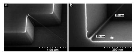
**Fig. 2.34** SEM images of the clamping point: (a) tilt-view showing clamping features and release, and (b) top-view showing width uniformity
