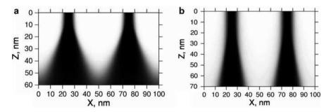
**Fig. 2.3** Electron beam broadening due to forward scattering in the resist at (a) 3 keV and (b) 10 keV of incident energy. Shown is a predicted cross-section of resist exposure for two parallel lines
