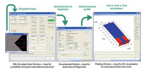
**Fig. 2.24** Screen-shots of the EBL simulator user interface demonstrating the procedures of graphic input, simulation of the exposure (*chain scission*) and development, and visualization of the results. Further details on the simulation tool can be found in Ref. [47]
