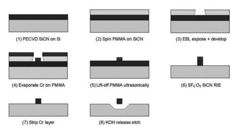
Fig. 2.21 Process flow outlining the steps used to fabricate doubly-clamped SiCN bridge resonators using a low voltage EBL and cold development process
