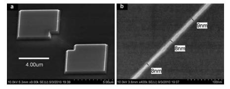
**Fig. 2.33** A sub-10 nm wide, 5 μm long doubly-clamped SiCN resonator: (a) overview image, and (b) a magnified image of the bridge
