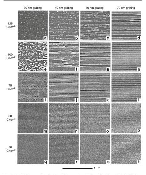
**Fig. 2.11** SEM images of 30, 40, 50, and 70 nm gratings fabricated in a 65-nm thick PMMA layer on a silicon substrate, with 10 keV exposure at various area doses. The gratings were developed for 5 s in a 1:3 MIBK:IPA solution at room temperature. The lateral size of all images is 1  $\mu$ m × 1  $\mu$ m [43]. The average area doses are related with the line doses by  $d_{area} = d_{line}l\lambda$ , where  $\lambda$  is the interline distance (grating pitch)
