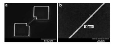
**Fig. 2.22** A sub-20 nm wide, 5  $\mu$ m long doubly-clamped SiCN resonator (a), and (b) a magnified image of the bridge showing a width of  $16 \pm 2$  nm [53]
