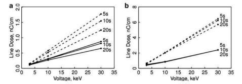
**Fig. 2.16** Applicable line dose windows for 70 nm pitch gratings in for 3, 10, and 30 keV exposure voltages and different durations of development at RT (a) and at  $-15^{\circ}$ C (b) [38]. The initial PMMA thickness was 55 nm. The meaning of the solid and dashed lines is as in Fig. 2.15
