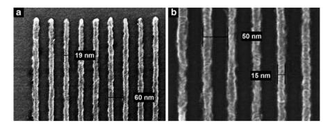
**Fig. 2.20** (a) 20 nm wide Cr lines in a 60 nm pitch grating, and (b) 15 nm wide Cr lines in a 50 nm pitch grating, both fabricated by 3 keV exposure of a single layer of PMMA 950 K resist, and developed at  $-15^{\circ}$ C
