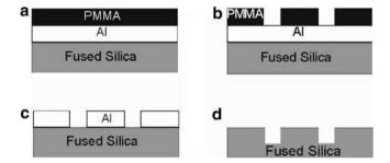
**Fig. 2.35** NIL mask fabrication schemes: (a) glass substrate is coated with Al and PMMA. (b) Patterns generated by e-beam exposure are realized in PMMA, (c) which is then transferred to the Al layer using dry etch with PMMA acting as the etch mask. (d) Patterns are then transferred to the glass substrate via glass etch process with the Al layer acting as hard mask. Finally the Al mask is removed from the fused silica surface
