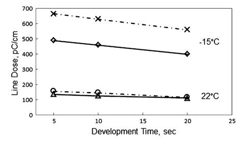
**Fig. 2.19** Comparison of dose windows for 3 keV exposure voltages developed at room temperature (*triangles and circles*) vs. at  $-15^{\circ}$ C (*diamonds and crosses*). The grating pitch is 70 nm and resist is 55 nm
