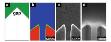
**Fig. 2.26** (a) Diagram of an alternative clamping point design with an optimized gap of 170 nm between resonator and pad, (b) the final dissolution profile compared with (c) a SEM image of the developed PMMA resist showing sharper corners compared to Fig. 2.25d, and (d) a SEM image of the released SiCN resonator clamping point [53]
