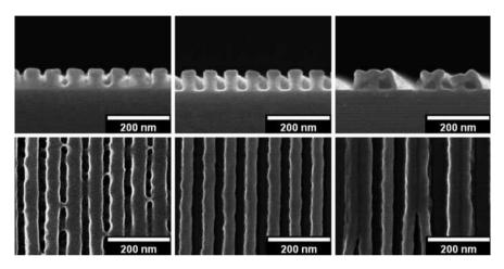
**Fig. 2.8** PMMA grating structures in cross-section (*top*) and plan view (*bottom*). Shown are underexposed/underdeveloped (*left*), quality structures (*middle*) and collapsed patterns (*right*) [31]
