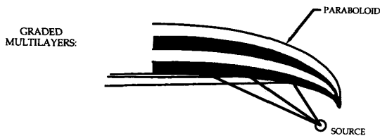
Fig. 15. Parabolic multilayer collimator with graded "d spacing" to allow for a changing angle of reflection.
