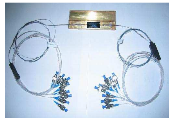
Fig. 5(b): Packaged LPWG device with 8-channel v-grooved fibre-array ribbon.
