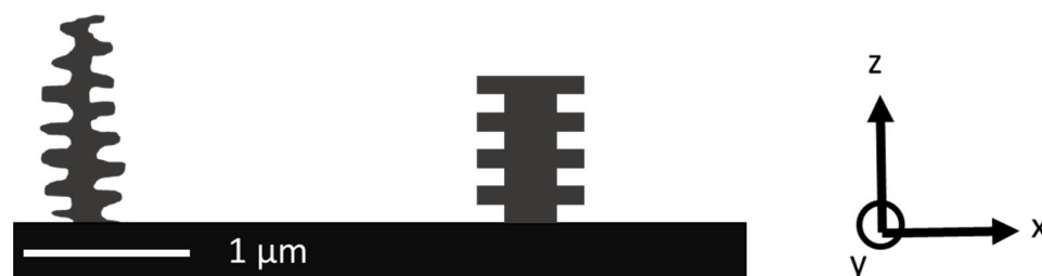
Figure 5. Sketch of a cross section of the tree-like nanostructures found on the wings of Morpho blue butterflies responsible for the metallic blue color. Left: exemplary sketch of the naturally occurring structure, Right: artificial design, that can be replicated using nanoimprinting.
