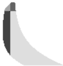
Fig. (3.7) A two-dimensional analysis of a six-mirror system in our class 37+. Horizontally, the curvature of the second surface varies, the curvature of the fourth surface alters vertically. The gray area is the unobstructed domain, wherein the different grayscales correspond to a specific class according to the classification by the sign of the powers of the mirrors.
