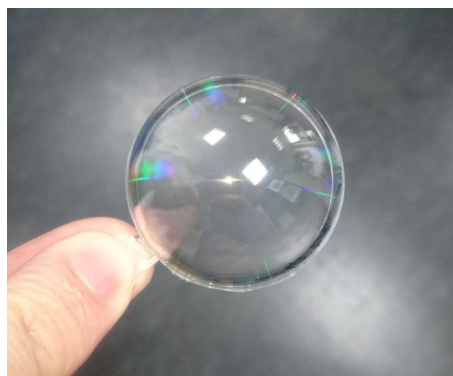
Figure 8. Photograph of a polymer hemisphere with moth-eye structures nanoimprinted on top. The high periodicity leads to diffraction colors when viewed under large angles. Details of the fabrication process can be found in [23].
