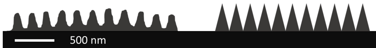
Figure 7. Moth-eye antireflective structures Left: Sketch of natural structures, Right: artificial idealized structure.
