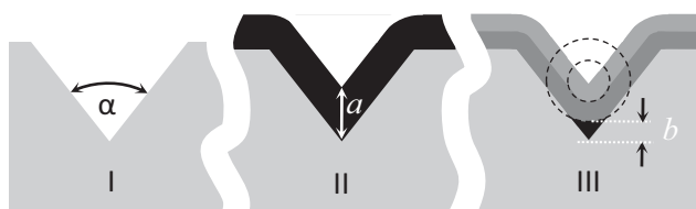
Figure 1. Corner Lithography concept (cross-sectional view): (I) V-groove template preparation, angle \alpha (II) deposition of conformal material, layer thickness t and thickness a in the corner (III) time controlled selective isotropic thinning by distance r leaving a nano feature of height b .
