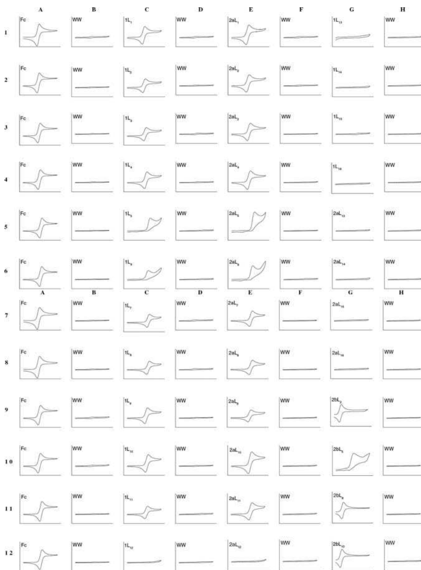
Fig. 14.20 Cyclic voltammetric array (potential axes range from -0.1 to 1.1 V vs. Ag/AgCl, current axes ranges from -80 to 180 nA) of samples in a microtiter plate as shown in Fig. 14.19; potential scan rate 0.5 V s^{-1} , all wells with 0.1 M NBu_4PF_6/CH_3CN electrolyte; reference wells with 0.5 mM Fc solution; sample wells with \sim 0.5 mM complex solution, wash wells (WW): electrolyte without redox active species; 200\mu m Pt disc electrode (Figure reprinted from Lindner et al. 71 Copyright Elsevier B.V. (2005))
