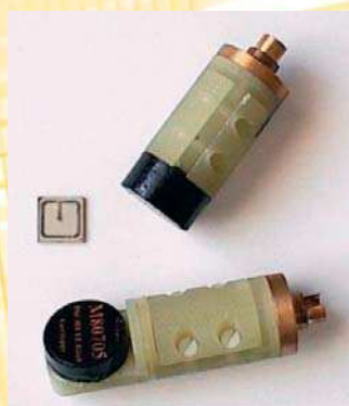
Fig. 3 Multilayer flux transformer on 10 mm x 10 mm \text{SrTiO}_3 substrate and encapsulated dc-SQUID magnetometers. The magnetometers are fixed on standard dc-SQUID packages (axial and 90°) designed for operation together with iMAG electronics (Tristan).
