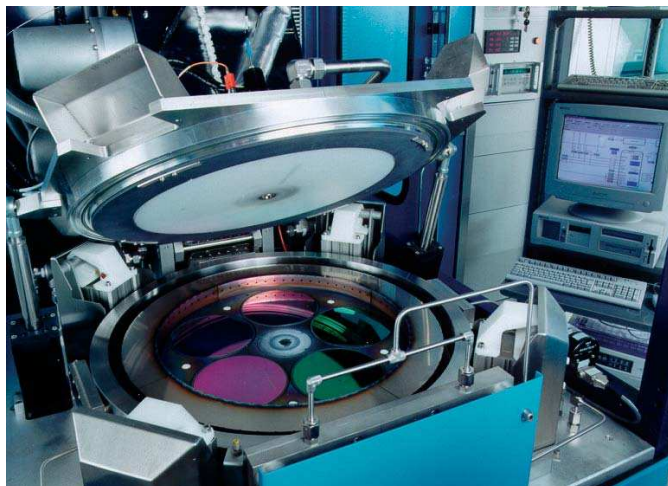
Fig. 2 MOCVD planetary reactor AIX-2600G3 from the AIXTRON AG, which can handle five 6" wafers simul- taneously
