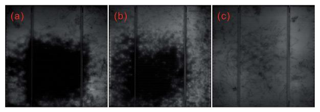
Fig. 32 EL images of BSi solar cells covered by different thickness of nano-rods: (a) 1  $\mu$ m; (b) 600 nm; and (c) 100 nm.<sup>209</sup> The black regions contain more defects, and correspond to non-uniform doped areas.
