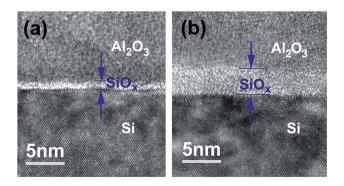
Fig. 45 TEM images of Al<sub>2</sub>O<sub>3</sub>/Si interfaces (a) in the as-deposited state; and (b) after 550  $^{\circ}\text{C}$  rapid thermal annealing. Reproduced with permission from ref. 286. Copyright 2011, AIP Publishing LLC.
