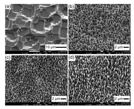
Fig. 14 SEM images of BSi samples fabricated via the PIII process at different reactive gas flow rates. (a)  $SF_6/O_2 = 3.5$ ; (c)  $SF_6/O_2 = 4.0$ ; and (d)  $SF_6/O_2 = 4.5$ . Reproduced by permission of Elsevier.
