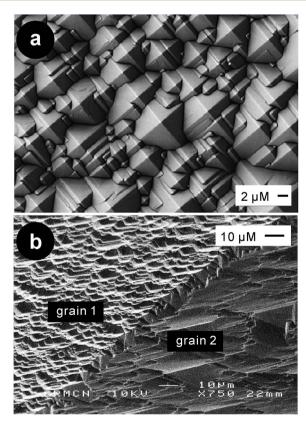
Fig. 27 SEM images of (a) a KOH etching textured (100) c-Si wafer; 182 and (b) anisotropic etching of a mc-Si wafer resulting in graindependent texturization. 152 Adapted by permission of Elsevier and SPIE.
