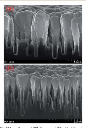
Fig. 38 700 nm Sputtered ITO film-coated BSi with different aspect ratios: (a) BSi composed of nano-rods with diameters  $\approx$  100 nm and lengths  $\approx$  500 nm; (b) BSi covered by nano-needles with diameters  $\approx$ 50 nm and lengths  $\approx 1.7 \,\mu\text{m}.^{214}$  Adapted by permission of SPIE.
