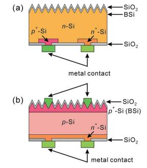
Fig. 53 (a) A schematic of a back-contact back-junction solar cell with a BSi front surface. 314 (b) A schematic of a back-junction solar cell with a BSi front surface and front surface field. 187
