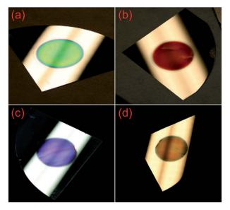
Fig. 5 Multi-layer porous silicon samples under the illumination of a white fluorescent lamp, exhibiting different colors: (a) green; (b) red; (c) purple; and (d) orange. Only a circular area of  $\sim$ 4 cm<sup>2</sup> has been electrochemically etched for each wafer and displays different colors, while the untreated area reflects white light. 68 Adapted by permission of Elsevier.
