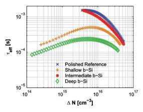
Fig. 48 Injection level dependent carrier lifetime of three BSi samples with different aspect ratios and a reference planar wafer. All samples are passivated with 100 nm Al<sub>2</sub>O<sub>3</sub>, and annealed in low-pressure Ar ambient at 425 °C for 30 min. Reproduced with permission from ref. 228. Copyright 2012, AIP Publishing LLC.
