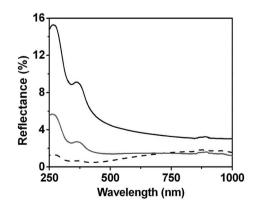
Fig. 9 Reflectance spectrum of hollow-needle arrays of different lengths, i.e., 2.1 μm (black solid line), 3.4 μm (gray solid line), and 7.1 μm (black dash line) in the UV-VIS-NIR region.99 Reproduced by permission of the Royal Society of Chemistry.
