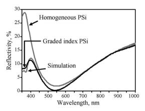
Fig. 4 Reflectance spectra of a homogenous porous silicon layer (80 nm thick, 75% porosity) and a gradient index porous silicon layer (100 nm thick). The later spectrum has an excellent match to the simulated reflectance of a porous layer with porosity gradient from 94% to 33%. Reproduced with permission from ref. 62. Copyright 2002, AIP Publishing LLC.
