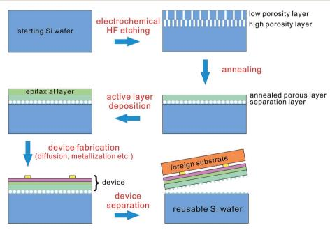
Fig. 41 Using porous silicon as a separation layer to produce thin film silicon solar cells.<sup>245</sup>
