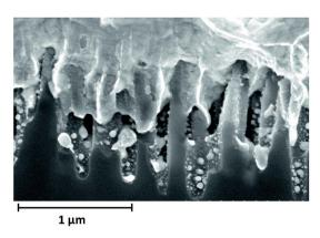
Fig. 33 SEM image of a BSi sample covered by printed front metal contact.<sup>220</sup> Reproduced by permission of Elsevier.
