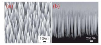
Fig. 16 SEM images of (a) a tilted top view and (b) a side view of a silicon nano-tip array, with a base diameter of ~200 nm and a height of 1600 nm.<sup>129</sup> Reproduced by permission of Nature Publishing Group.
