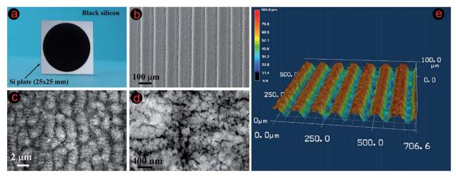
Fig. 52 (a) A photography of laser treated BSi; (b) SEM image of the micro-grooved BSi; (c) and (d) correspond to the zoomed-in SEM images, showing the micro- and nano-scale surface texture, respectively; (d) A 3D optical image of the micro-grooved BSi.<sup>304</sup> Adapted by permission of Elsevier.
