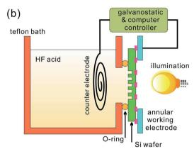
Fig. 1 Typical experimental setups for electrochemical HF etching of: (a) p-Si; and (b) n-Si.55,56
