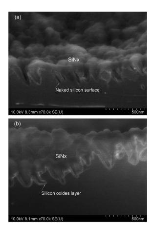
Fig. 44 SEM images of BSi coated with (a) 80 nm  $SiN_x$ ; and (b) 20 nm thermal oxide and 60 nm  $SiN_x$ .<sup>207</sup> Reproduced by permission of John Wiley & Sons, Inc.
