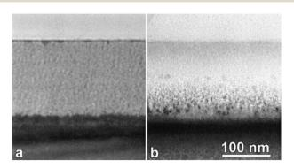
Fig. 2 TEM images of (a) electrochemically and (b) stain etched porous silicon, with a thickness of ~150 nm. The porosity is uniform in the electrochemical case, but possesses a gradual transition in the stain etched case. 63 Reproduced by permission of the Electrochemical Society.
