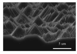
Fig. 51 A micro- and nano-dual scale surface texture on a (100) wafer.<sup>224</sup> Reproduced by permission of the Electrochemical Society.
