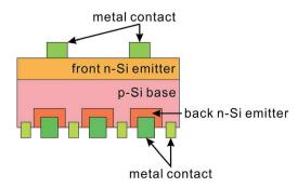
Fig. 40 Tandem n<sup>+</sup>-p-n<sup>+</sup> solar cell using laser treated BSi.<sup>241</sup>
