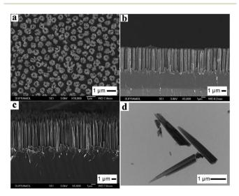
Fig. 8 SEM images of (a) top view and (b) side view of a hollow silicon columnar array, formed via Aq-assisted chemical etching; and (c) side view of this array after a quick RIE process, demonstrating hollow needle-like structures, with a height of  $\sim$ 7.1  $\mu$ m; (d) TEM image of the hollow-needles isolated from the silicon substrate.99 Reproduced by permission of the Royal Society of Chemistry.
