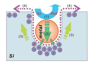
Fig. 7 An illustration of the metal-assisted chemical etch process: (1) the reduction of an oxidative agent (such as H<sub>2</sub>O<sub>2</sub>) catalyzed by a noble metal particle; (2) the injection of the holes generated during the reduction reaction, into the silicon substrate, with the highest hole concentration underneath the metal particle; (3) the migration of holes to silicon sidewalls and surfaces; and (4) the removal of oxidized silicon via HF.92
