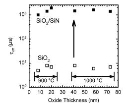
Fig. 49 Comparison of the effective lifetime in a low resistivity p-Si wafer with only SiO<sub>2</sub> passivation (open squares) and with a SiO<sub>2</sub>/SiN<sub>x</sub> stacked passivation layer. The SiO<sub>2</sub> thickness varies according to the growth temperature (900 or 1000 °C) and growth time (5-63 min), while the thickness of  $SiN_x$  is fixed at 60 nm.<sup>263</sup> © IOP Publishing. Reproduced by permission of IOP Publishing. All rights reserved.
