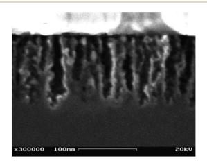
Fig. 3 SEM image of a gradient index porous silicon, with a thickness of ~100 nm. Reproduced with permission from ref. 62. Copyright 2002, AIP Publishing LLC.
