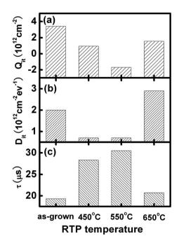
Fig. 46 Evolution of (a) interfacial fixed charge density,  $Q_{it}$ ; (b) density of interfacial states,  $D_{it}$ ; and (c) effective carrier lifetime,  $\tau$ , for Al<sub>2</sub>O<sub>3</sub> passivated p-Si wafers annealed at different temperatures via rapid thermal processing (RTP). Reproduced with permission from ref. 286. Copyright 2011, AIP Publishing LLC
