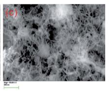
Fig. 25 SEM images of porous silicon formed through the FFC-Cambridge process by directly reducing a  $2 \mu m SiO_2$  precursor at E = -1.0 V and t=20 min. (a) Side and (b) top views of silicon nano-nucleation; and (c) top view of silicon nano-fibres. Scale bar =200 nm. <sup>174</sup> Reproduced by permission of the Electrochemical Society.
