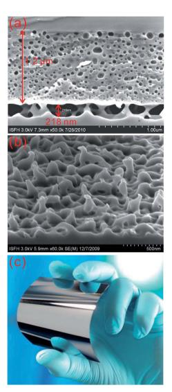
Fig. 42 SEM images of (a) a low porosity silicon layer after epitaxial deposition (top), sitting on top of a silicon substrate (bottom) via a high porosity separation layer (middle); and (b) the tilted view of the separation layer after the top layer is lifted off. (c) Photograph of the top layer (30  $\mu m$  thick, 9  $\times$  9 cm<sup>2</sup> large).<sup>246</sup> Adapted by permission of Elsevier.
