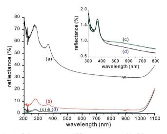
Fig. 15 Reflectance spectra of BSi samples produced by PIII etching, as a function of  $SF_6/O_2$  gas ratio: (a)  $SF_6$  (black); (b) 3.5 (red); (c) 4.0 (green); and (d) 4.5 (blue). The inset shows magnified spectra of cases (c) and (d).118 Adapted by permission of Elsevier.
