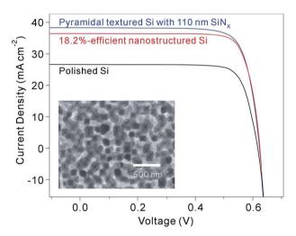
Fig. 30 J-V curves of 18.2%-efficient nanostructured BSi, polished silicon and pyramid-textured silicon with a SiN<sub>x</sub> antireflection coating under AM1.5 illumination. Inset: top-view SEM image of the BSi solar cell.<sup>32</sup> Reproduced by permission of Nature Publishing Group.
