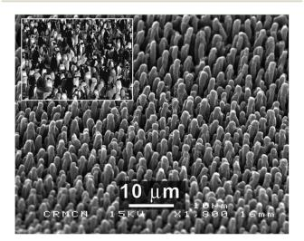
Fig. 22 SEM image of penguin-like silicon microstructures created by fs-laser irradiation; the inset shows a real penguin colony.151 Reproduced by permission of Elsevier.
