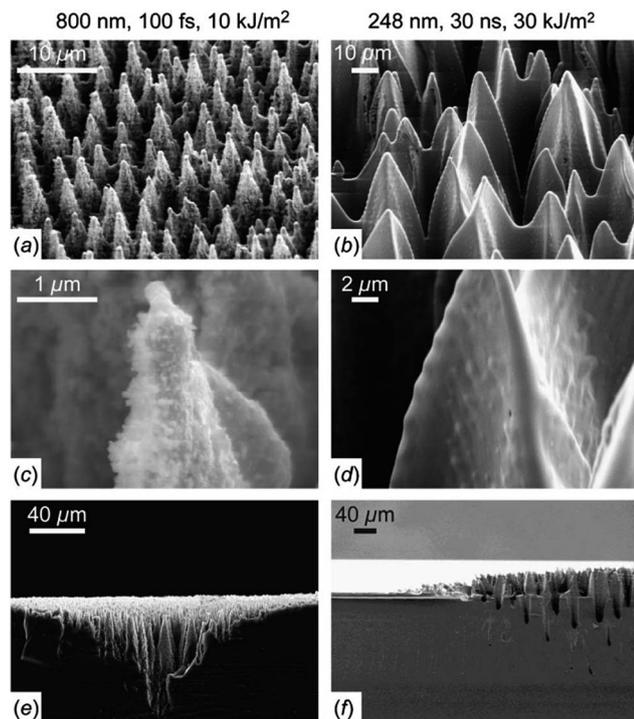
Fig. 20 SEM images of laser-treated silicon surfaces in a SF<sub>6</sub> environment with [(a), (c) and (e)] fs-laser, and [(b), (d) and (e)] ns-laser. (e) and (f) show the side views of the snapped samples. Reproduced with permission from ref. 142. Copyright 2004, AIP Publishing LLC.
