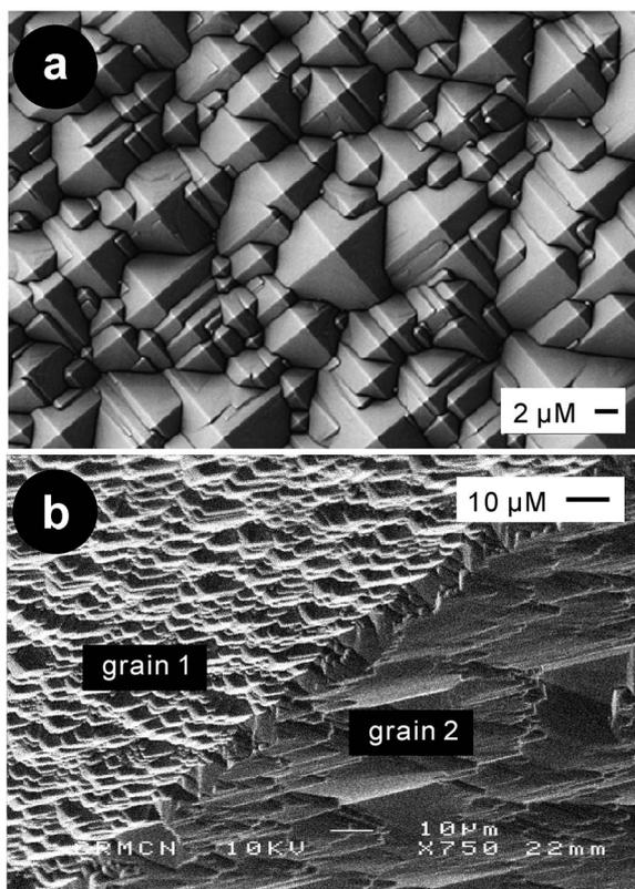
Fig. 27 SEM images of (a) a KOH etching textured (100) c-Si wafer,<sup>182</sup> and (b) anisotropic etching of a mc-Si wafer resulting in grain-dependent texturing.<sup>152</sup> Adapted by permission of Elsevier and SPIE.
