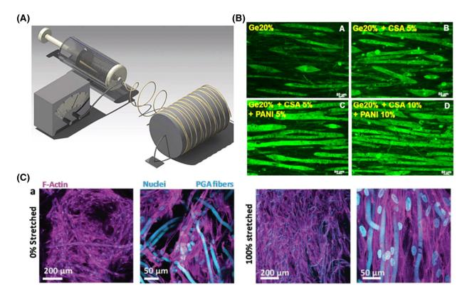
**FIGURE 8** (A) A schematic illustration of a conventional electrospinning set-up. Reprinted with permission from Ref. [152] Copyright (2016) Wiley. (B) Myotube formation on aligned electrospun in different composition conditions. Reprinted with permission from Ref. [166] Copyright (2017) American Chemical Society. (C) Confocal images of fibroblasts cultured over non-stretched and stretched PGA scaffolds. Reprinted with permission from Ref. [176] Copyright (2018) Wiley
