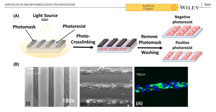
**FIGURE 1** (A) A schematic illustration of the fabrication of micropatterned constructs using photolithography. (B) Photolithographic approach to generate cellular micropatterns (i) Crosslinked chitosan pattern after 180 s of UV exposure (315–400 nm), (ii) neonatal rat cardiomyocytes after 8 days of culture, (iii) cardiac troponin I (green) expressed from the patterned cardiomyocytes. Reprinted with permission from Ref. [38] Copyright (2006) Elsevier Ltd.
