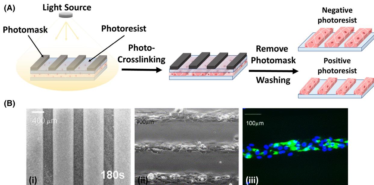
**FIGURE 1** (A) A schematic illustration of the fabrication of micropatterned constructs using photolithography. (B) Photolithographic approach to generate cellular micropatterns (i) Crosslinked chitosan pattern after 180 s of UV exposure (315–400 nm), (ii) neonatal rat cardiomyocytes after 8 days of culture, (iii) cardiac troponin I (green) expressed from the patterned cardiomyocytes. Reprinted with permission from Ref. [38] Copyright (2006) Elsevier Ltd.
