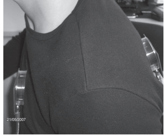
FIGURE 11: Setup for the channel-loss measurement, setup between the front and the back of a human chest.
