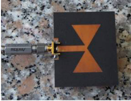
FIGURE 10: Antenna prototype for the channel model verification.
