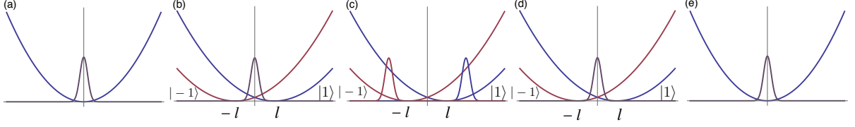
FIG. 5. Illustration of one stage of the splitting protocol for gravimetry. Shown are the spin dependent harmonic trapping potentials along the \hat{z} direction and the one dimensional spatial wave function for the resonator as a function of z . This protocol is repeated M(K, k) times for each value of the qubit resonator coupling \lambda_k = 2^k \lambda_0 , for k = 0, \dots, K where \lambda_0 is a minimal value of the coupling. (a) At t < 0 the resonator is prepared in the ground motional state with an rms width z_0 and frequency \omega . The qubit is not coupled to the resonator ( \lambda_k = 0 ). (b) At time t = 0 the qubit is prepared in the superposition state |+_x\rangle and the interaction \lambda_k is turned on. The trapping potential is now state dependent with minima located at \pm l = \pm \lambda_k z_0 / \omega . (c) After half an oscillation period, the state dependent motional wave packets are maximally separated by a distance 4l . (d) After a full oscillation period, the wave packets recombine, localised at the origin with the accumulated gravitationally induced phase \phi_k mapped onto the qubit. (e) The interaction is turned off and the qubit is measured. For [M(K, k)] rounds the qubit is measured in the basis \{| \pm_x \rangle basis and for the other [M(K, k)] rounds in the basis \{(|1\rangle + e^{-i\pi/M(K,k)}| - 1\rangle) / \sqrt{2}, (e^{i\pi/M(K,k)}|1\rangle - | - 1\rangle) / \sqrt{2}\} providing an estimate \hat{\phi}_k of the phase \phi_k . After the last stage the resonator returns to a ground state of the trapping potential.
