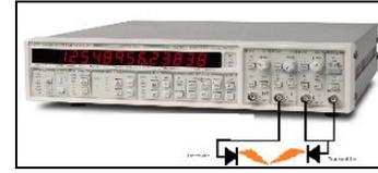
Fig. 10. Jitter Measurement Setup.
