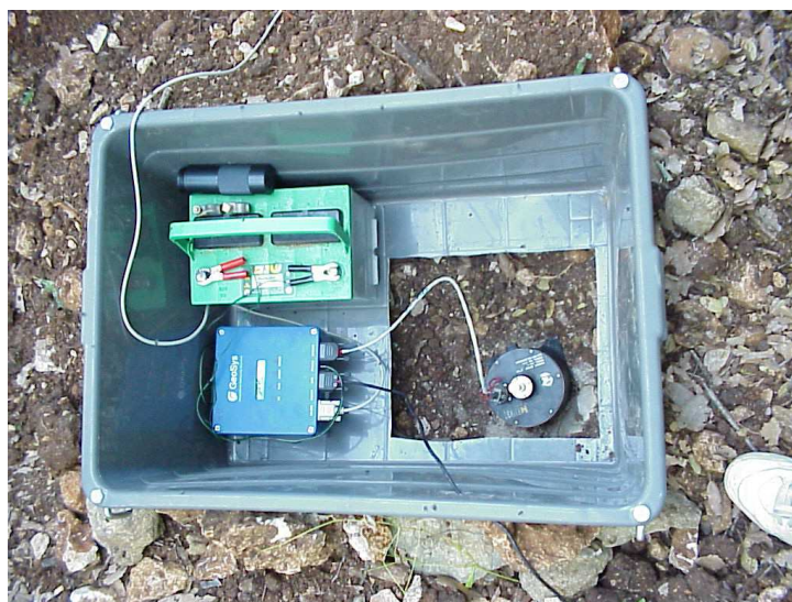
Figure 7.12 A simple field installation. A plastic box has been placed directly on the ground. The sensor is placed in the cut out hole. Inside is also the battery and recorder. The cable going out is for the GPS. After installation, soil was put up around the sides and insulation was put on top of the lid. The sensor is a Kinemetrics Ranger 1 Hz seismometer (Table2.2) and the recorder a GeoSig GBV316 (Table 5.3).
