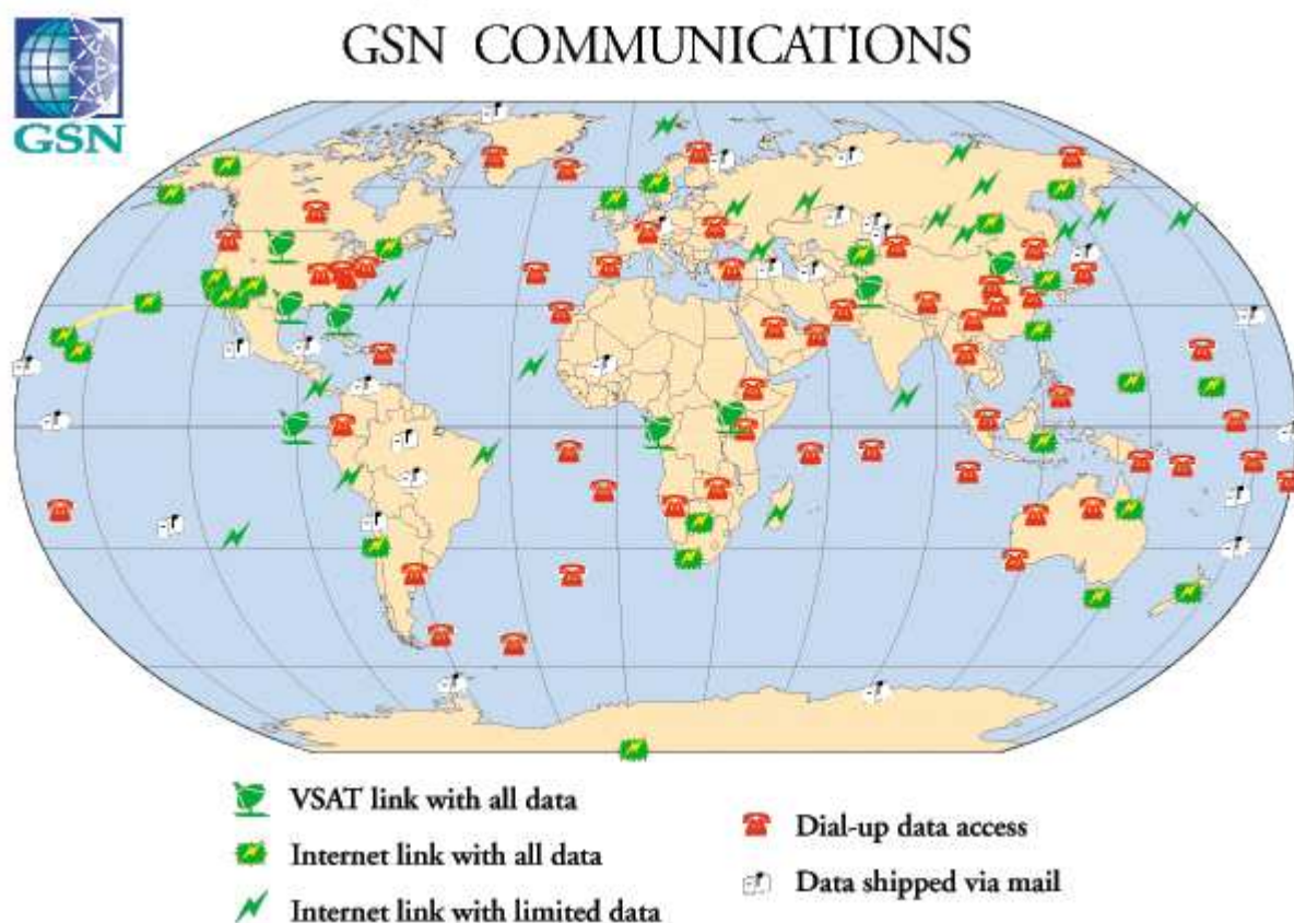
Figure 8.21 Communication to GSN stations 2001. VSAT is satellite connection. VSAT and internet have real time connections and potentially all data can be downloaded, while the dial up stations on transmit a limited amount on data. Figure from IRIS home page.
