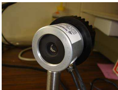
Fig. 1. A temperature-controlled pyroelectric transfer-standard radiometer head.
