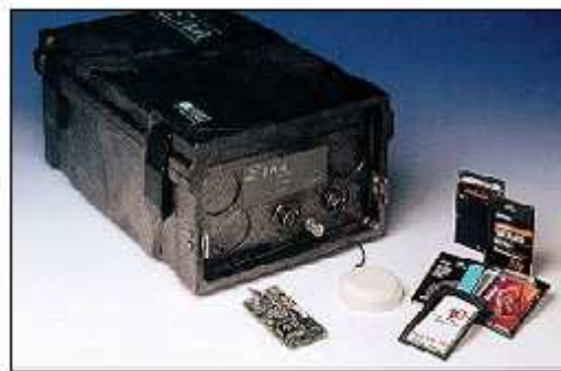
Figure 5.13. Example of a recorder make specifically for strong motion, the Kinemetrics Etna. The round white box in front of the recorder is the GPS antenna and the PCMCIA cards are seen to the right.
