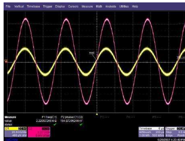
Figure 8.3: OPA227 A_v=50\text{dB} @ 2.2 kHz
