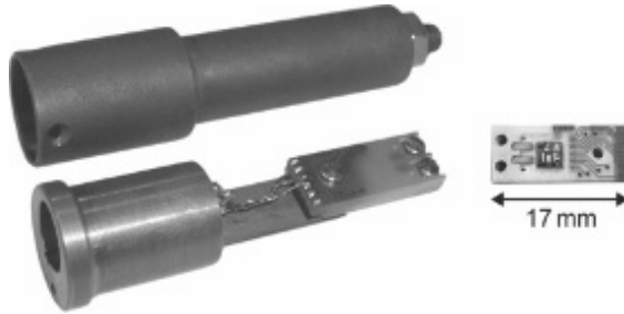
Figure 8.12 Example of a commercial SQUID package. The superconducting connection to the input coil is realized via screw contacts. For low-noise operation, the SQUID carrier is enclosed by a Nb shield. On the left side, the socket for the wiring to the room temperature electronics is visible. Picture courtesy of Magnicon GmbH, Hamburg.
