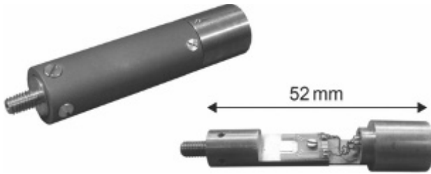
Figure 8.20 Sensor module of a commercial MFFT. The multiloop gradiometer in Fig. 8.13b is used to measure the thermal noise currents in the temperature sensor; a solid block of high-purity Cu. Picture courtesy of Magnicon GmbH, Hamburg.
