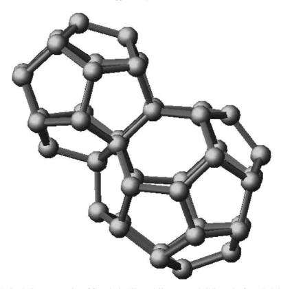
Fig. 1. Symbolic representation of face sharing  $Si_{20}$  and  $Si_{24}$  cages as building unit of type-I clathrates.
