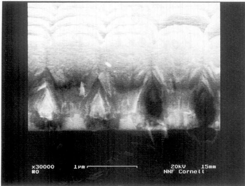
Fig. 3. Electron micrograph showing side view of a sample with similar features as in Fig. 2 after backfilling with 600 nm of Ti metal.
