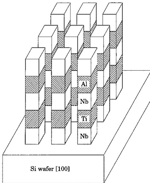
Fig. 1. Schematic diagram showing the columns of alternating superconductor/normal metal cubes after etching. Top cubes represent residual e-beam resist.
