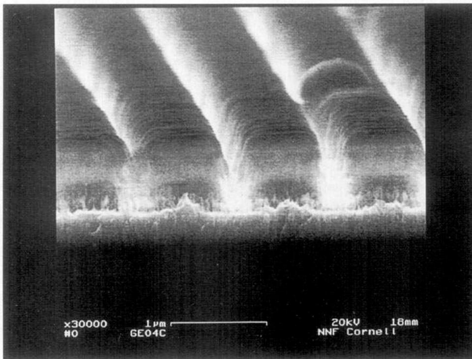
Fig. 2. Electron micrograph of a three-layer sample after etching. Sample is viewed from the side to illustrate vertical sidewall etching. Features shown are  $0.5 \mu\text{m}$  squares with  $0.5 \mu\text{m}$  gap spacing.
