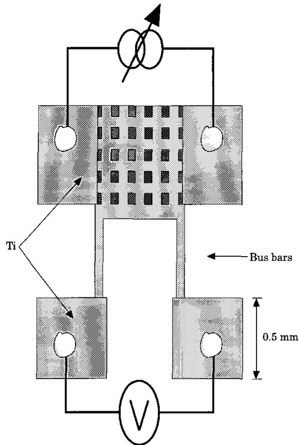
Fig. 4. Schematic diagram of the array voltage and current contact pad arrangement.
