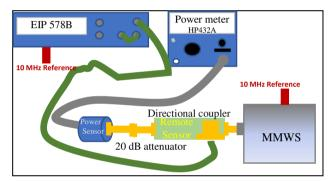
Fig. 6. Measurement setup of MMWS1.
