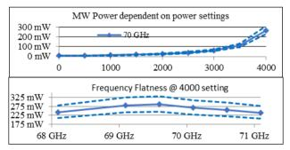
Fig. 7. Measurement results of MMWS.
