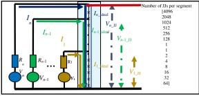
Fig. 8. Connection diagram of DACs & arrays of JJs.
