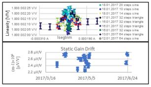
Fig. 13. Static linearity measurement results.
