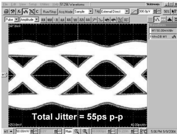
Fig. 20. Tx eye diagram after 36 in of FR-4 and two connectors at 6.25 Gb/s.
