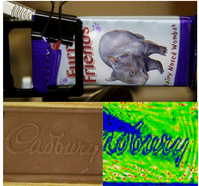
Figure 6. Optical photos of the wrapped chocolate bar with a metallic blade inserted (upper picture) and the text on the chocolate (lower left), and THz image of the chocolate bar (lower right).
