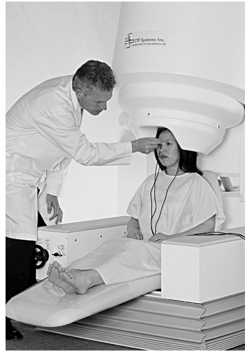
Fig. 7. System for MEG with 275 sensor channels and 29 reference channels (courtesy CTF Systems, Inc.).
